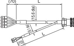
[Servomotor Connector]<br>Straight plug:<br>N/MS3106B24-11S<br>(Japan Aviation Electronics Industry, Ltd.)<br>Cable clamp:<br>N/MS3057-16A<br>(Japan Aviation Electronics Industry, Ltd.) |
