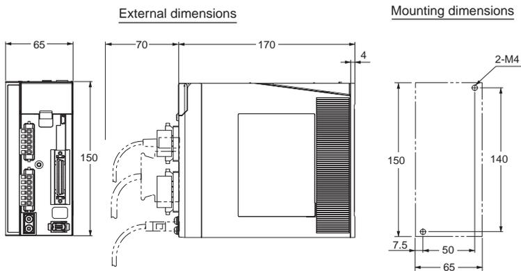
Single-phase/Three-phase 200 VAC R88D-KP10H/-KP15H (900W to 1.5kW)
