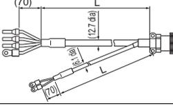
[Servomotor Connector]<br>Straight plug:<br>N/MS3106B20-18S<br>(Japan Aviation Electronics Industry, Ltd.)<br>Cable clamp:<br>N/MS3057-12A<br>(Japan Aviation Electronics Industry, Ltd.) |
