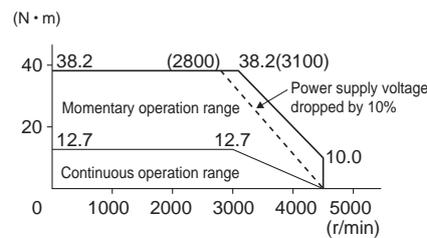
**Note 1:** The continuous operation range is the range in which continuous operation is possible. Continuous operation at the maximum speed is also possible. However, doing so will reduce the output torque.
