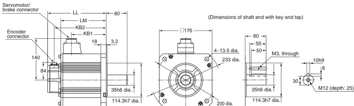
**Note:** The standard models have a straight shaft. A model with a key and tap is indicated by adding "S2" to the end of the model number. Models with an oil seal are indicated with O at the end of the model number. The motor dimensions do not change.
