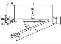
[Servomotor Connector]<br>Straight plug:<br>N/MS3106B20-18S<br>(Japan Aviation Electronics Industry, Ltd.)<br>Cable clamp:<br>N/MS3057-12A<br>(Japan Aviation Electronics Industry, Ltd.)   |
