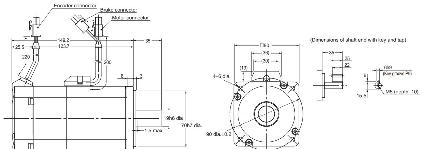
**Note:** The standard models have a straight shaft. A model with a key and tap is indicated by adding "S2" to the end of the model number. Models with an oil seal are indicated with O at the end of the model number. The motor dimensions do not change.
