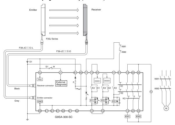
S1: External test switch KM1 and KM2: Magnetic Contactors M: 3-phase motor
