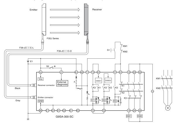
S1: Reset switch (momentary action switch) Timing Chart
