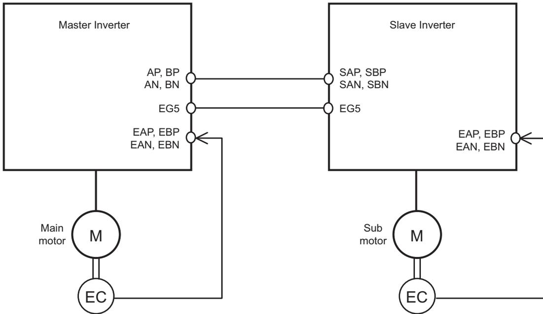
For the Inverter (master Inverter) on the main motor side, you can select either the speed control or pulse train position control mode.
