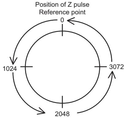
Motor shaft viewed from motor shaft load side
