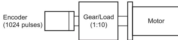
When the motor-to-encoder rpm ratio is 1:10, set the following data.
