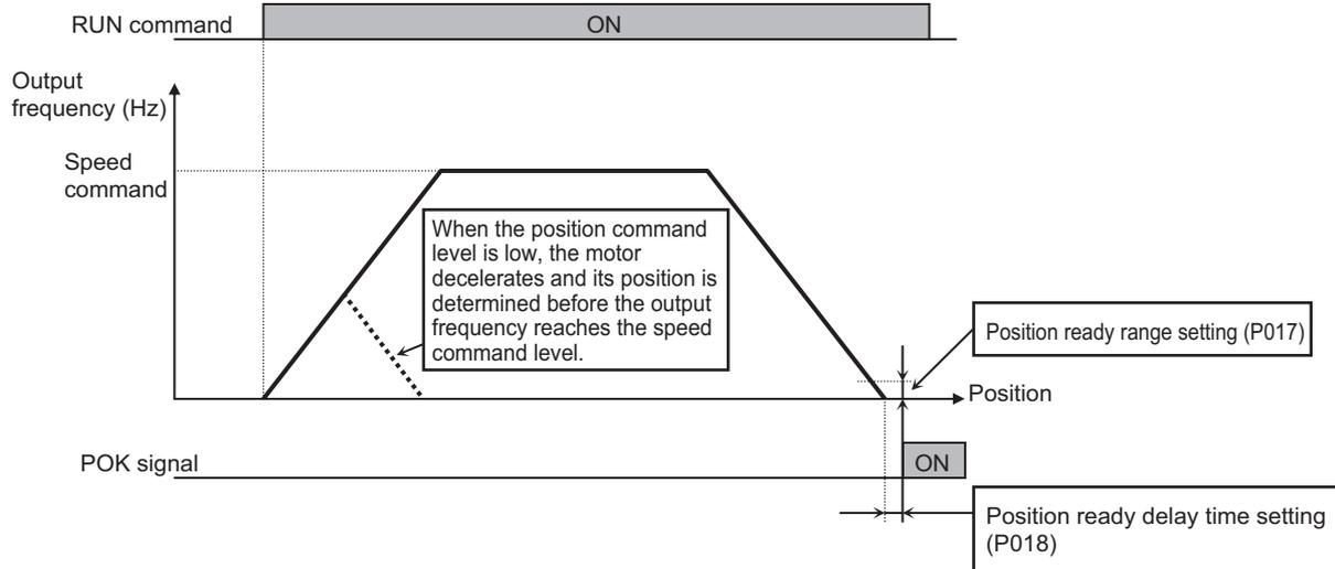
In the absolute position control mode, the Inverter moves to the target position according to the following parameter settings, and is then set in the position servo lock status.
