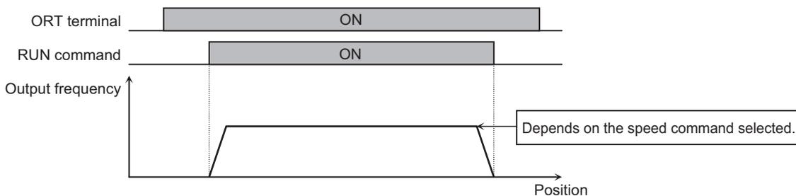
\* If the Inverter control circuit (Ro, To) is turned on, teaching is enabled.
