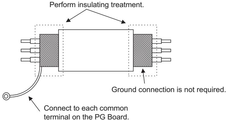
Note 3: Separate the wiring from that of the main circuit and/or the relay control circuit. If they have to be crossed, be sure to cross them at right angles.
