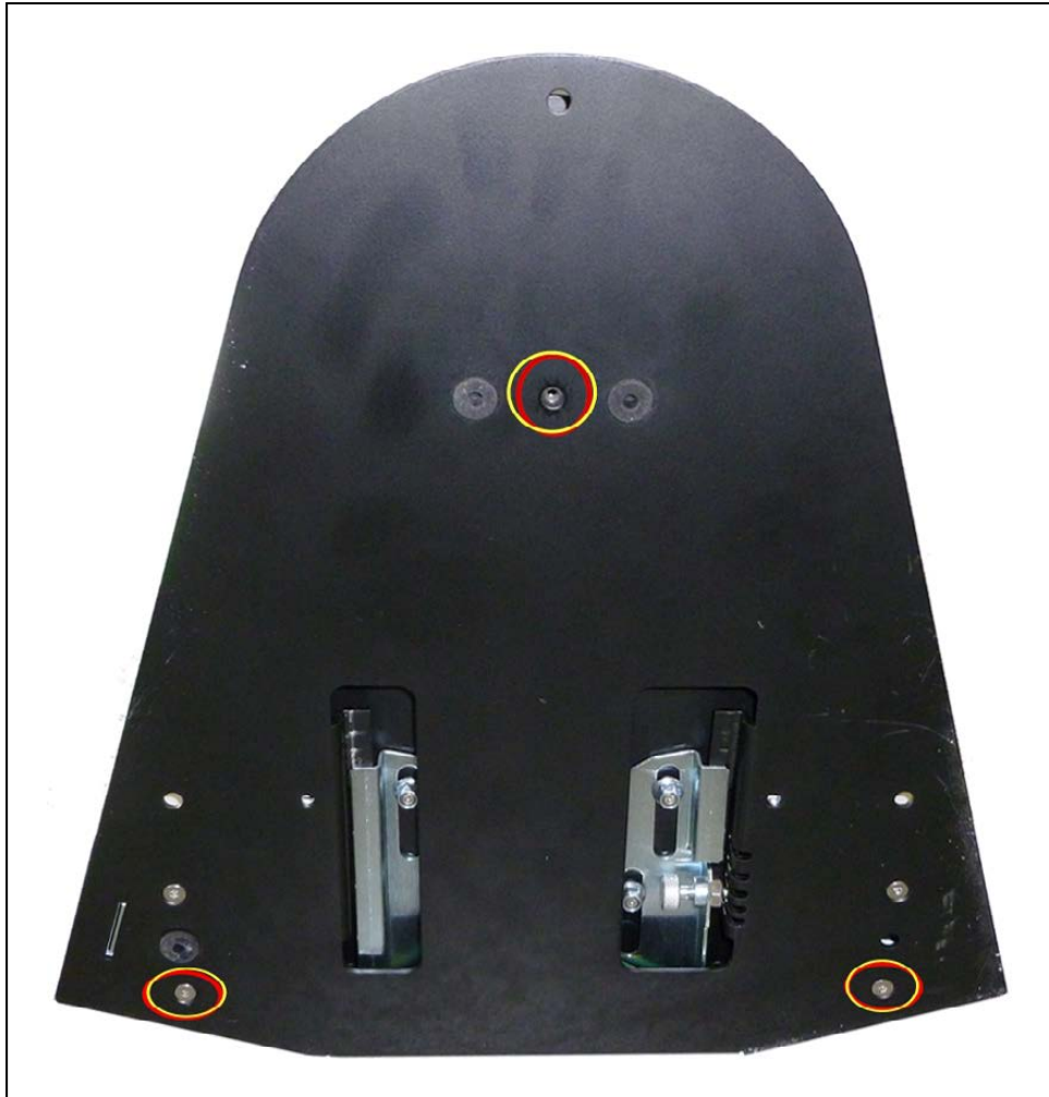
Figure 3-21. Underside of Docking Station Foot, Showing Screw Locations
