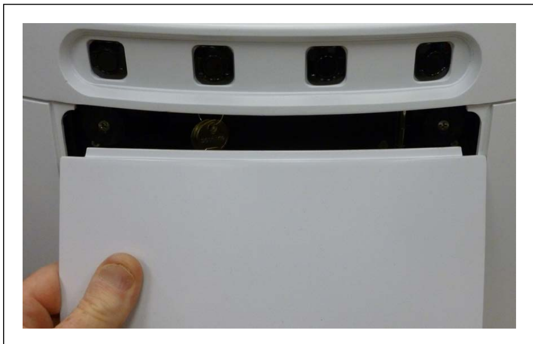
Figure 3-14. Lowering the Battery Door Platform Skin
