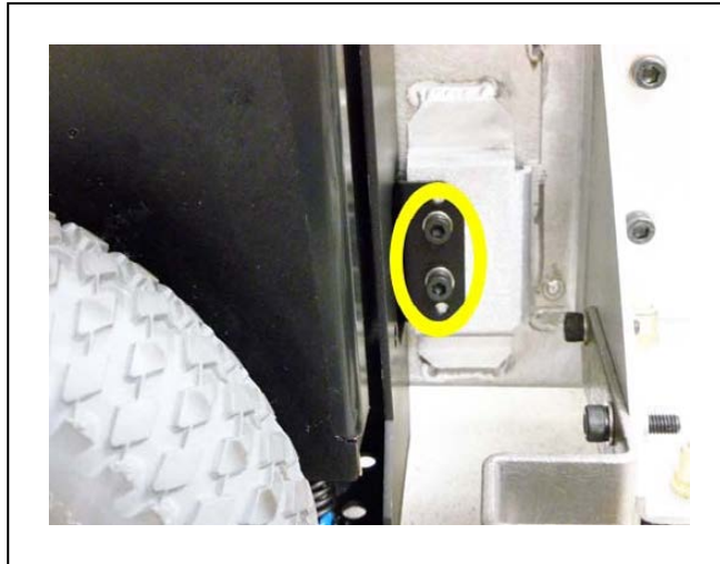
Figure 8-16. Mounting Screws at Bottom-Right of Drive Assembly
