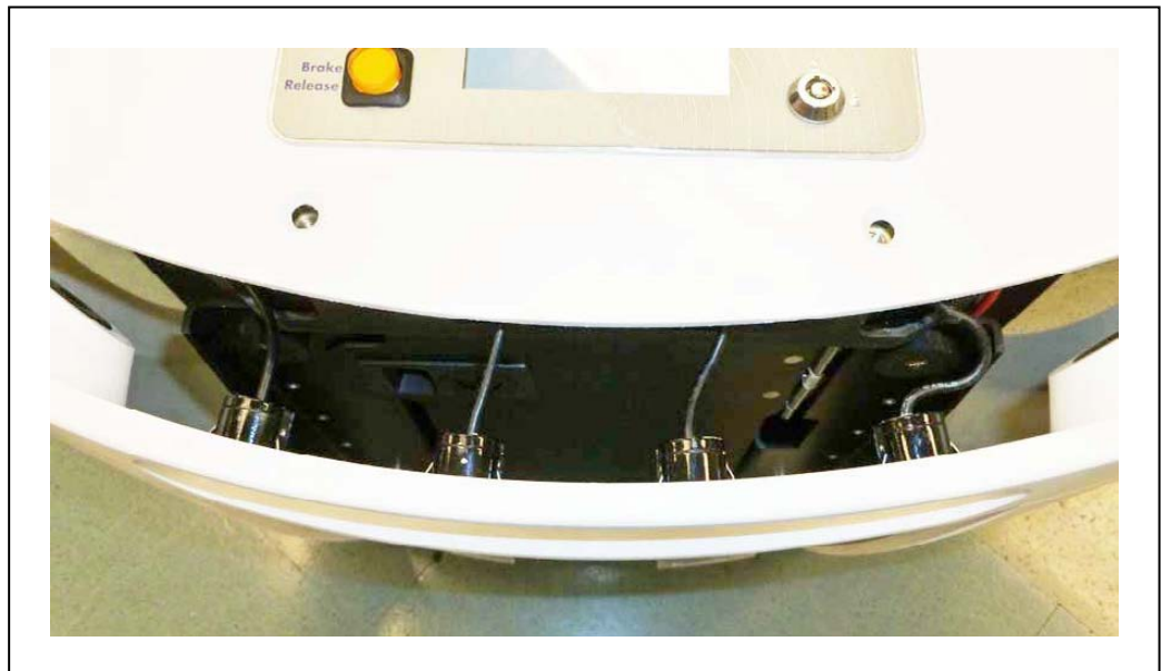
Figure 8-20. Sonar Leads, with Connectors Still in Chassis
