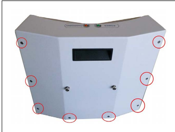
Figure 8-9. Docking Station Rear Cover Screws (8 of 10)
