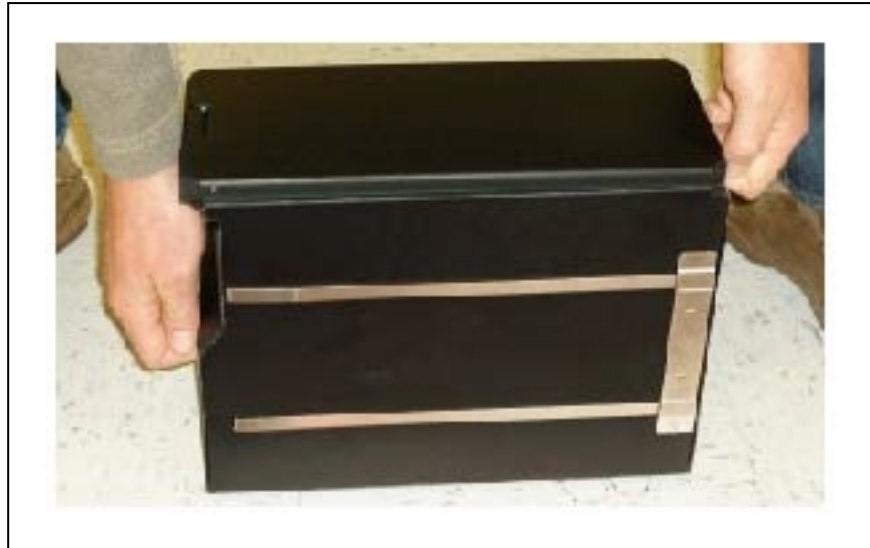
Figure 3-16. Lifting the Battery
