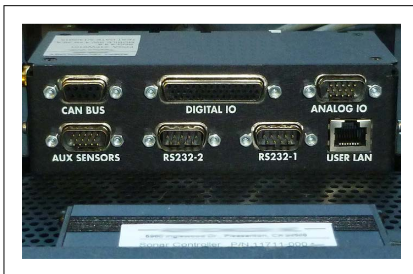
Figure 9-10. Upper Front of Core, Showing RS232 Ports
