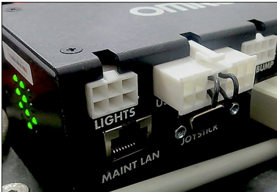
Figure 3-18. E-Stop Jumper on LD Platform Core
