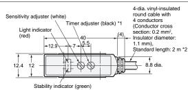
\*1. Not applicable to Sensors with timer adjusters (E3S-AT11 and E3S-AT31). \*2. The E3S-AT11 or E3S-AT31 has three conductors.
