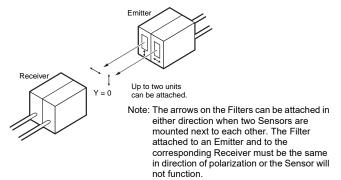
The arrow printed on the cover indicates the direction of polarization. By attaching the Filters opposite to each other in polarization to the Emitters and the Receivers in rows, mutual interference can be prevented (in any case, the Filter attached to an Emitter and to the corresponding Receiver must be the same in direction of polarization or the Photoelectric Sensor will not function).
