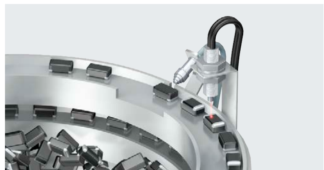
Air blower output during chip's front/rear detection
