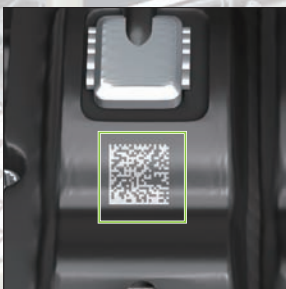
Reading direct part marks
