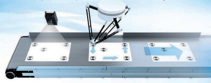
**Step 1 - camera** Camera detects all calibration marks. **Step 2 - robot** Robot moves to the calibration marks. The offset to the camera is registered through the encoder value. Step 3 - system Camera, conveyor, robot and encoder are automatically aligned.
