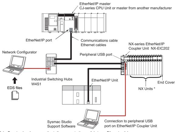
**Note:** Do not make a loop connection in the communications path between Ethernet switches. \* Refer to *Configuration Unit* on page 8 for the NX Units that can be connected to the NX-series EtherNet/IP Coupler Unit.
