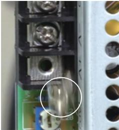
Previous The screw is loosened and dropped by vibration...
