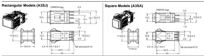
Note: Unless specified, a tolerance of  $\pm 0.4$  mm applies for all dimensions. Use a mounting panel thickness of 1 to 4 mm.
