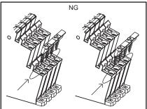
Some arrow marks are added to the top of short bar as figures below. These arrow marks indicate the direction toward the relays mounted on the G2RV-SR/G3RV-SR series. When installing the short bar into G2RV-SR/G3RV-SR, short bar shall be installed as the arrow marks heading to the mounted relays.
