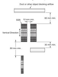
\* When five or more are installed, install with 10 mm space between each.
