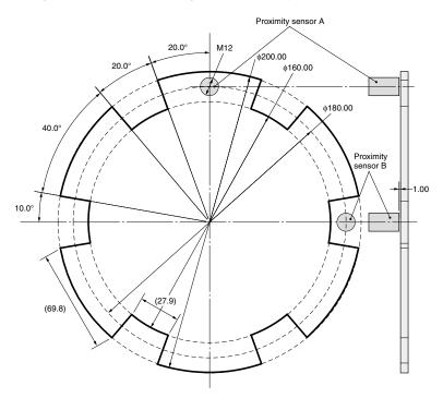
When installing proximity sensors in the vertical direction to the cogwheel surface, note that the height of cogwheel teeth should not be affected by surrounding metal products. For details in influence of surrounding metal, see the E2E Catalog.
