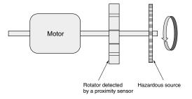
Perform a risk assessment for entire equipment including the conditions of use to implement safety measures. (For example, attaching a protective cover around a cogwheel)
