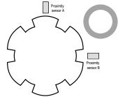
Install proximity sensors so that one of them is turned ON when the rotation of cogwheel stops. Install one proximity sensor on the center line of the concavity width, and the other on the center of the convexity width so that one of the proximity sensors will be turned ON when the rotation of the cogwheel stops.
