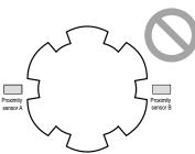
With this installation, both proximity sensors are turned OFF when the rotation of the cogwheel stops. If both sensors are turned OFF for more than 1 second, G9SX-LM $\square$  will detect it as an error.
