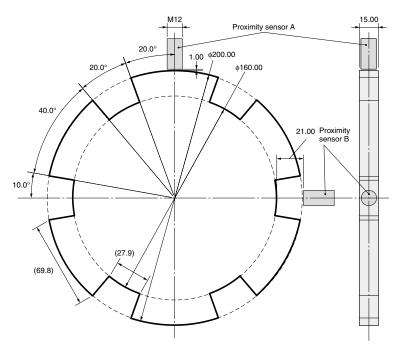
The diagram below shows a design when proximity sensors are installed in the vertical direction to the cogwheel surface.
