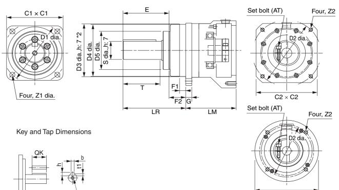
\*2. With the R88G-HPG50 $\Box$ , the height tolerance is 8 mm (D3 dia., h: 8).
