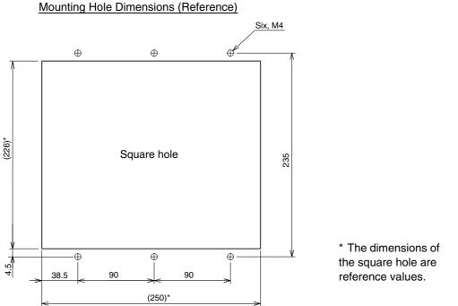
Dimensions for front panel mounting are references values that provide leeway.
