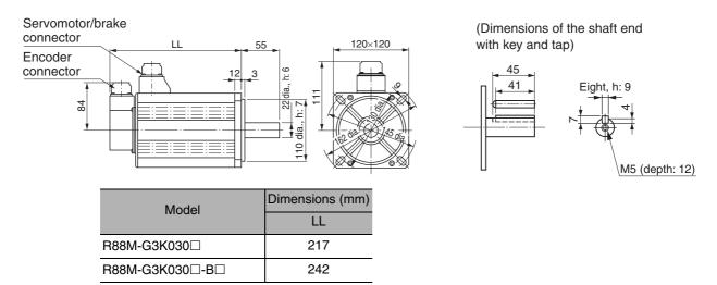
**Note** The standard models have a straight shaft. Models with a key and tap are indicated with "S2" at the end of the model number.
