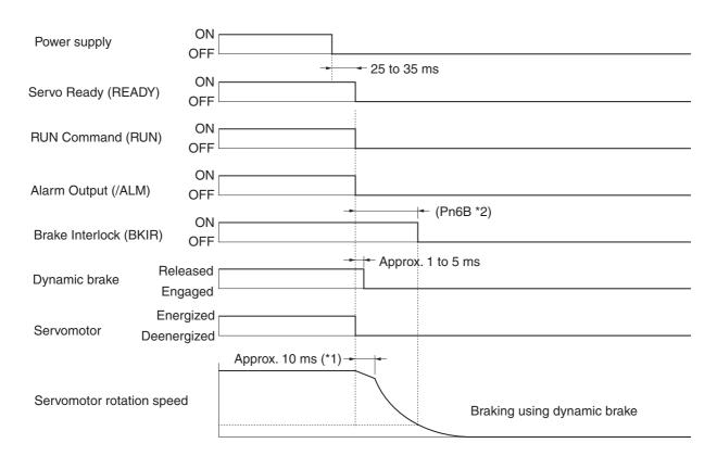
\*1. After the Servomotor is deenergized, it will rotate by inertia for approximately 10 ms until the dynamic brake operates.
