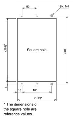
Dimensions for front panel mounting are references values that provide leeway.
