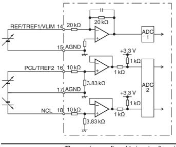
Precautions for Correct Use The maximum allowable input voltage is  $\pm 10$  V for each input. The VR must be 2 k $\Omega$  with B characteristics and 1/2 W minimum. R must be 200  $\Omega$  and 1/2 W minimum.
