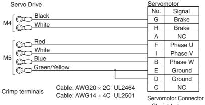
ervomotor Connector Straight plug: N/MS3106B20-18S (Japan Aviation Electronics) Cable clamp: N/MS3057-12A (Japan Aviation Electronics)
