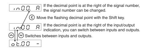
The following procedure can also be used to switch between inputs and outputs.
