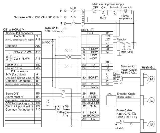
\*1. The I/O bits for the CS1W-HCP22 depend on the memory allocations in the CIO Area. Change the wiring according to the allocations.
