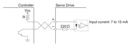
• Select a resistance R value so that the input current will be from 7 to 15 mA. Refer to the following table.
