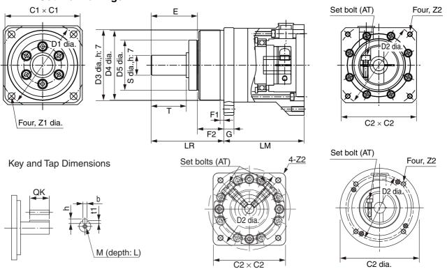
For the R88G-HPG11B Series, two set bolts are positioned at  $90^{\circ}$  from each other.
