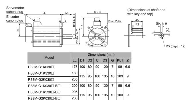
**Note** The standard models have a straight shaft. Models with a key and tap are indicated with "S2" at the end of the model number.
