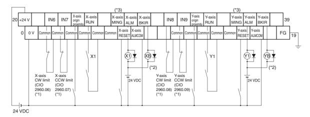
\*1. CW and CCW limit input signals can also be input through Input Units. The bits for the CW/CCW limit inputs in the CJ1M are as follows: CW: A540.08, CCW: A540.09 for pulse output 0 and CW: A541.08, CCW: A541.09 for pulse output 1. For example, the flag for the CW limit input (A540.08) can be controlled with an output from the ladder diagram using a bit allocated to the actual input (CIO 2960.06) on the Input Unit, as shown below. Example:
