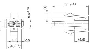
Connector housing: 172157-1 (Tyco Electronics AMP KK) Contact socket: 170366-1 (Tyco Electronics AMP KK) Panel Mounting Hole
