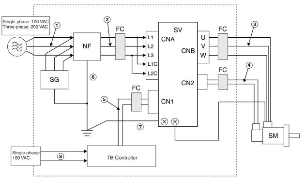
\*1. For models with a single-phase power supply input (R88D-GTA5L/-GT01L/-GT02L/-GT04L/-GT01H/-GT02H/-GT04H/-GT08H), the main circuit power supply input terminals are L1 and L3.
