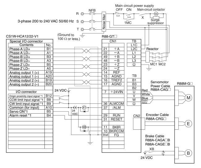
\*1. The I/O bits for the CS1W-HCA12/22 depend on the memory allocations in the CIO Area. Change the wiring according to the allocations.
