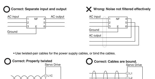
• Separate power supply cables and signal cables when wiring.
