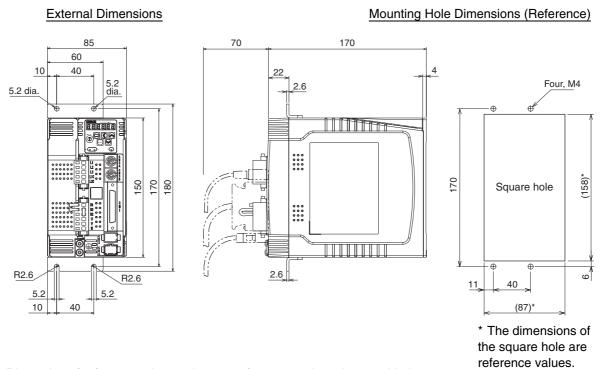
Dimensions for front panel mounting are references values that provide leeway.
