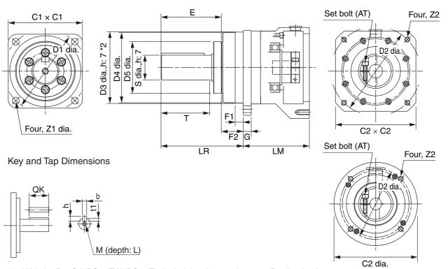
\*2. With the R88G-HPG50 $\Box$ /-HPG65 $\Box$ , the height tolerance is 8 mm (D3 dia., h: 8).
