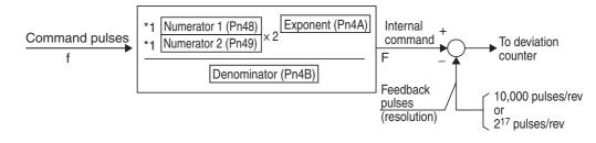
\*1. Numerator 1 or Numerator 2 is selected using the Electronic Gear Switch Input (GESEL: CN1 pin 28).
