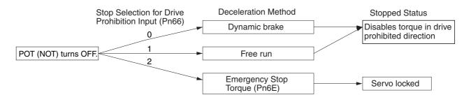
While the Forward Drive Prohibit Input (POT) is OFF, the Servomotor cannot be driven in the forward direction, but it can be driven in the reverse direction. Conversely, while the Reverse Drive Prohibit Input (NOT) is OFF, the Servomotor cannot be driven in the reverse direction, but it can be driven in the forward direction.
