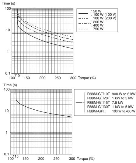
When the torque command = 0, and a constant torque command is continuously applied after three or more times the overload time constant has elapsed, the overload time t [s] will be: t [s] = – Overload time constant [s] × log<sub>e</sub> (1 – Overload level [%] / Torque command [%])<sup>2</sup>
