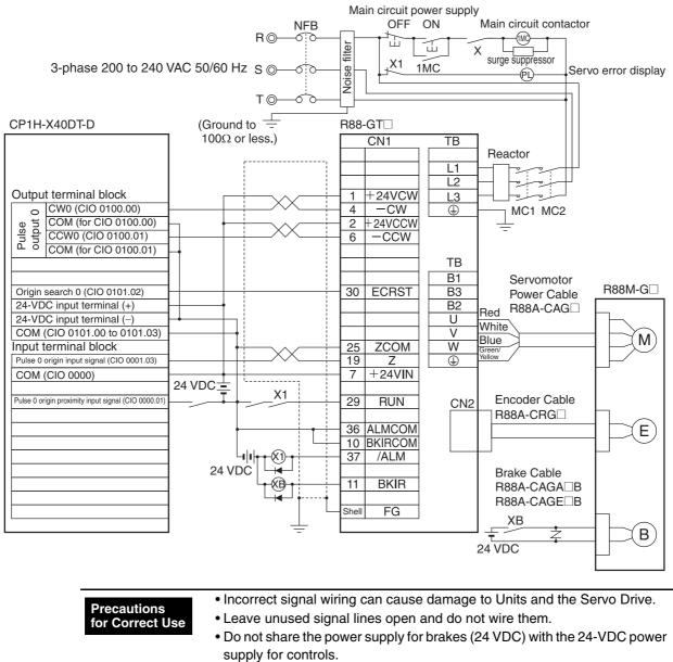
• The diode recommended for surge absorption is the RU 2 manufactured by Sanken Electric or the equivalent.
