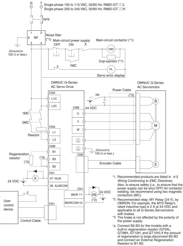
\*5. The models GTA5L to GT02L and GT01H to GT04H do not have a built-in regeneration resistor. If the amount of regeneration is large, an External Regeneration Resistor must be connected to B1-B2.
