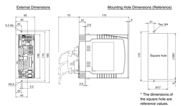
Dimensions for front panel mounting are references values that provide leeway.
