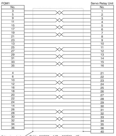
Crimp terminal — Cable: AWG28 × 14P + AWG28 × 4C
