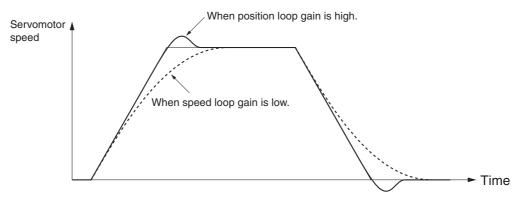
• If the speed loop gain and position loop gain are optimally set, the Servomotor operation for the command will be delayed 2/Kp at acceleration and delayed 3/Kp at deceleration.
