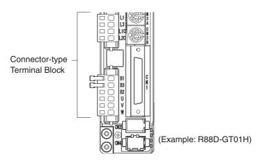
1. Remove the Terminal Block from the Servo Drive before wiring. The Servo Drive will be damaged if the wiring is done with the Terminal Block in place.
