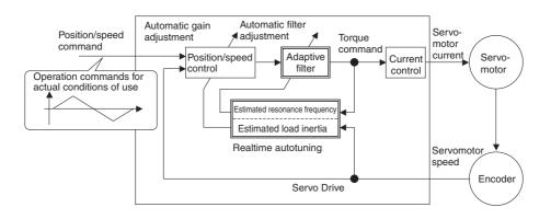
• Realtime autotuning may not function properly under the conditions described in the following table. If realtime autotuning does not function properly, use normal mode autotuning or manual tuning.
