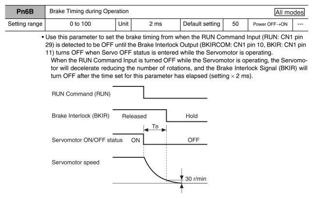
"TB" in the above figure is the brake timing during operation (setting  $\times$  2 ms) or the time until the speed of the Servomotor falls to 30 r/min or lower, whichever is shorter.
