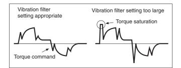
• The vibration filter setting is restricted by the following equation. 10.0 Hz – Vibration frequency  $\leq$  Vibration filter setting  $\leq$  Vibration frequency
