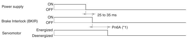
\*1. The time from turning OFF the brake power supply to the brake engaging is 100 ms max. If using the Servomotor on a vertical axis, take this delay into account and set the Brake Timing when Stopped (Pn6A) so that the Servomotor is deenergized after the brake has engaged.
