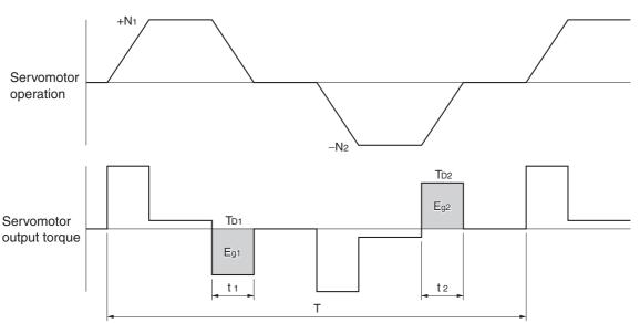
• In the output torque graph, acceleration in the positive direction is shown as positive, and acceleration in the negative direction is shown as negative.
