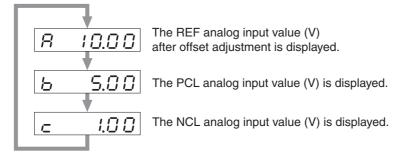
Note: The displayed value will not be accurate if the voltage exceeds  $\pm 10$  V.
