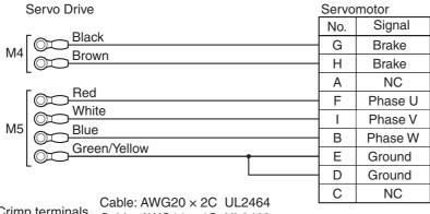
Crimp terminals Cable: AWG20 × 2C UL2464 Cable: AWG14 × 4C UL2463
