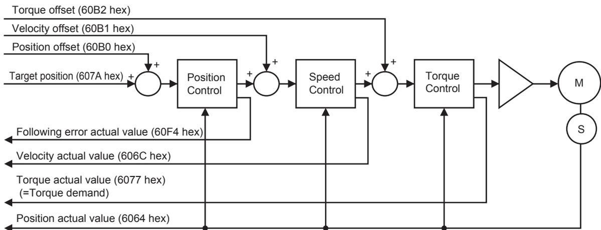
The following diagram shows the configuration of the control function of the Cyclic synchronous position mode.
