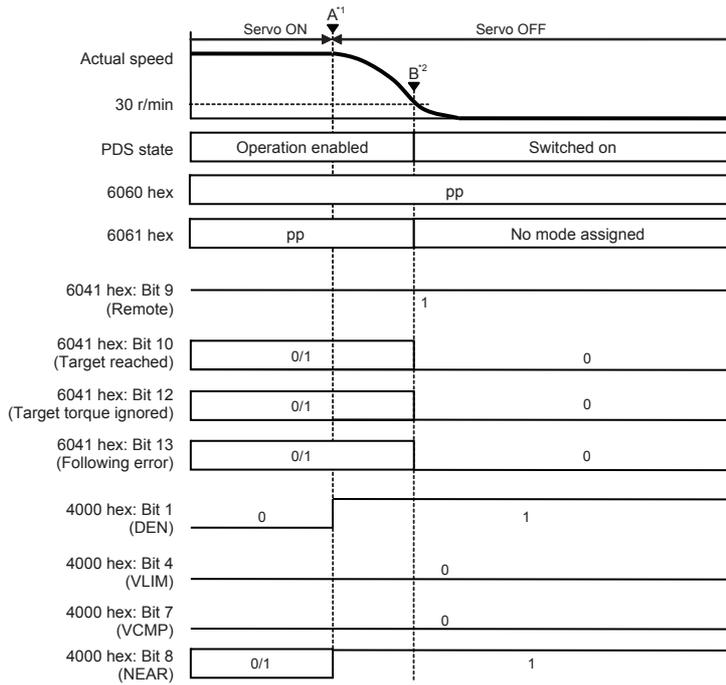
\*1 When the servo is turned OFF, a deceleration stop starts and 6061 hex continues to show the same mode as the mode of operation (pp) specified in 6060 hex.
