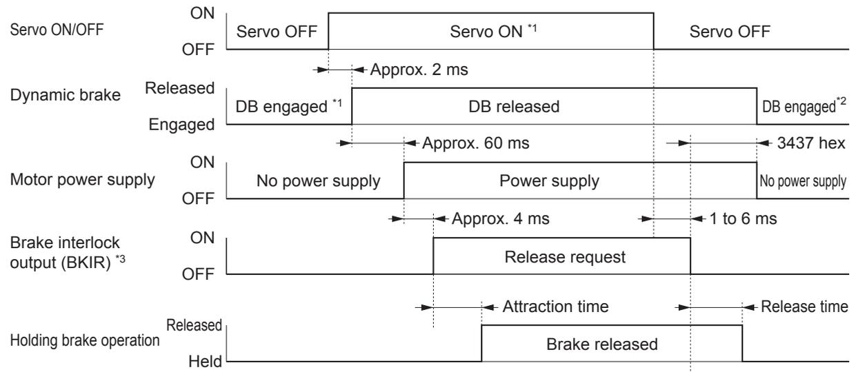
\*1 The servo does not turn ON until the motor rotation speed drops to approx. 30 r/min or below.
