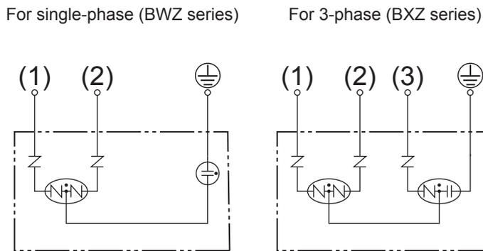
**Noise Filter for the Brake Power Supply**
