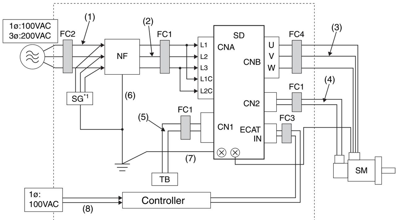
\*1 Not required for single-phase models with a 100-VAC input.
