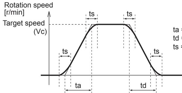
$$t_a = V_c / \text{Maximum motor rotation speed} \times 3312 \text{ hex} \times 1 \text{ ms}$$
