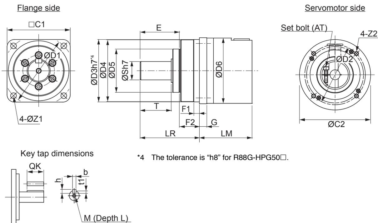
● For 2,000-r/min Servomotors (400 W to 1 kW)
