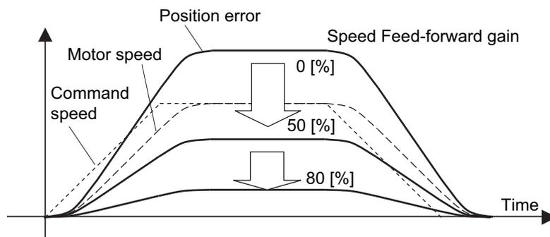
The position error in the range of constant speed becomes smaller as the speed feed-forward gain increases.
