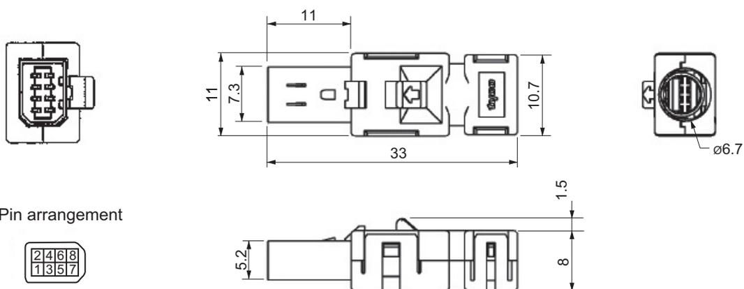
**Note** The recommended cable is a 6-core shielded cable with a wire size of AWG30 to AWG26 and a finished outer diameter of 6.7 mm or less.
