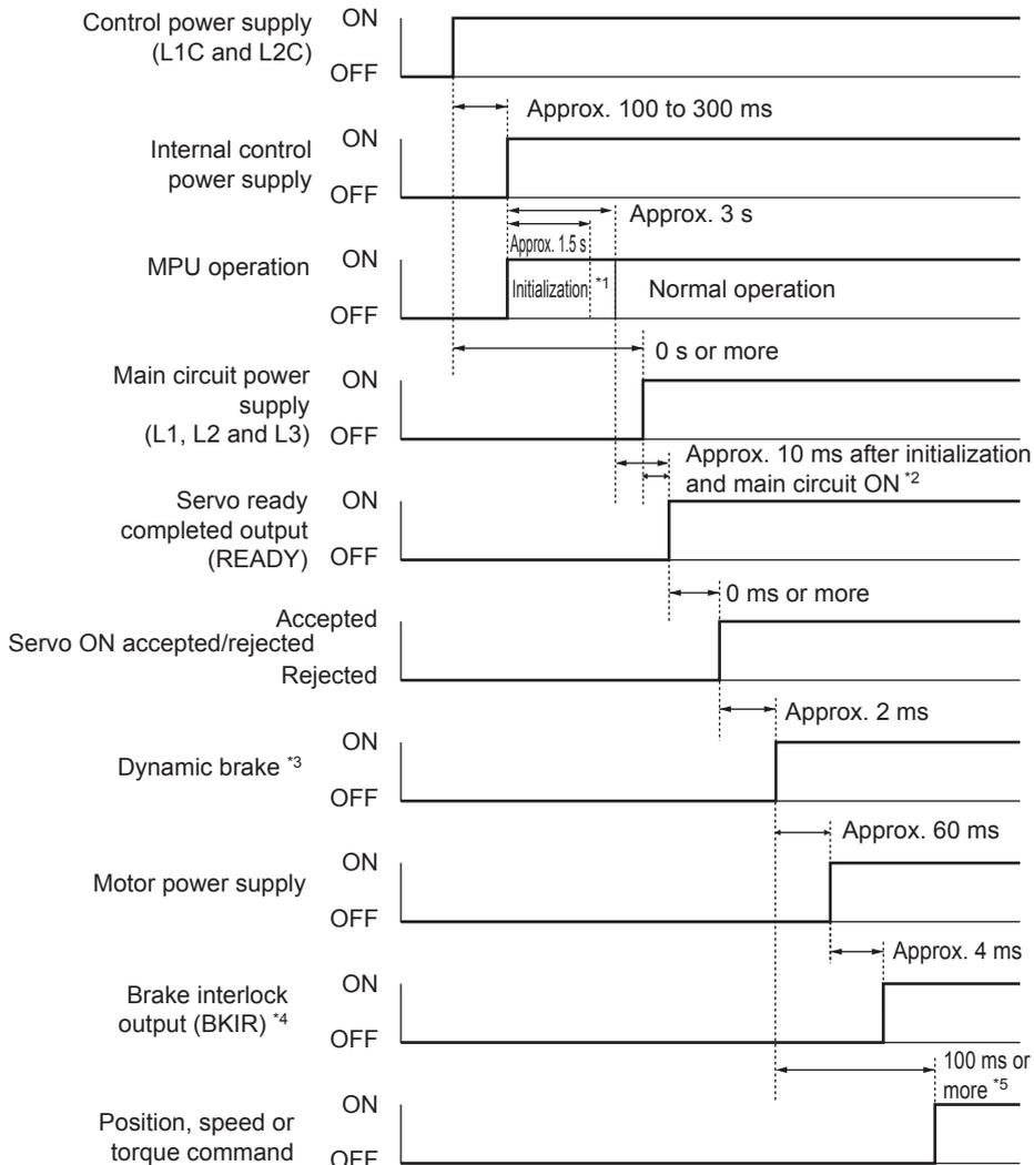
\*1 Once the internal control power is established, the protective function starts working about 1.5 s after the MPU starts initializing itself. Be sure that all I/O signals that are connected to the Servo Drive, especially the Forward/Reverse Drive Prohibition Input (POT/NOT), the Origin Proximity Input (DEC), the external encoder input, are stable before the protective function starts working. The period can be extended by setting the Power Supply ON Initialization Time (3618 hex).
