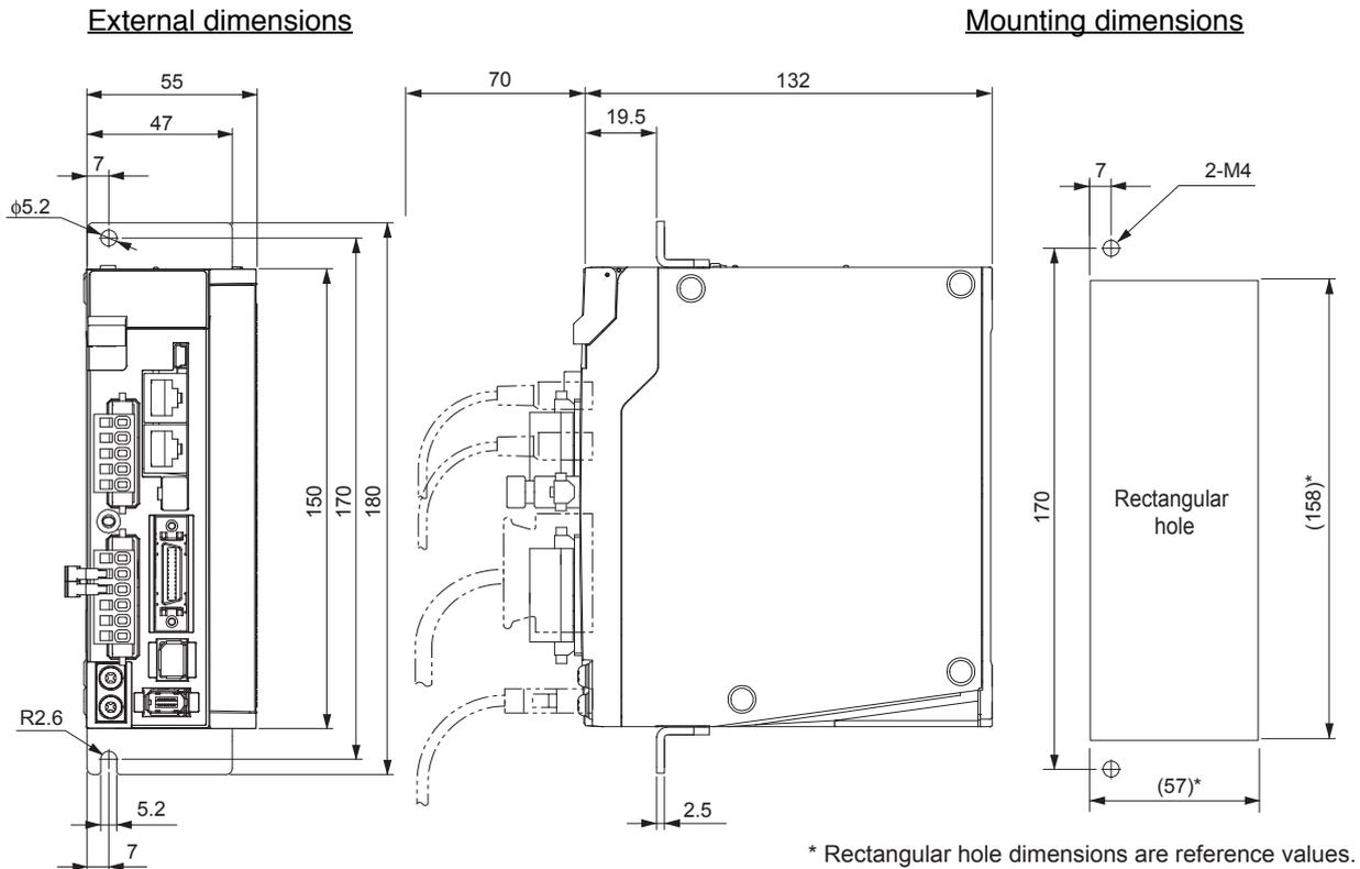
**Single-phase/3-phase 100 VAC: R88D-KN04L-ECT (400 W)**
