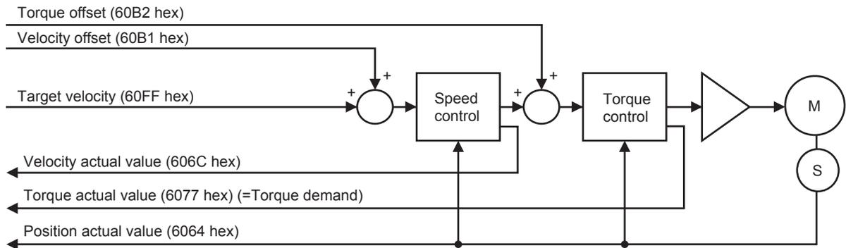
The following diagram shows the control function configuration of the Cyclic synchronous velocity mode.
