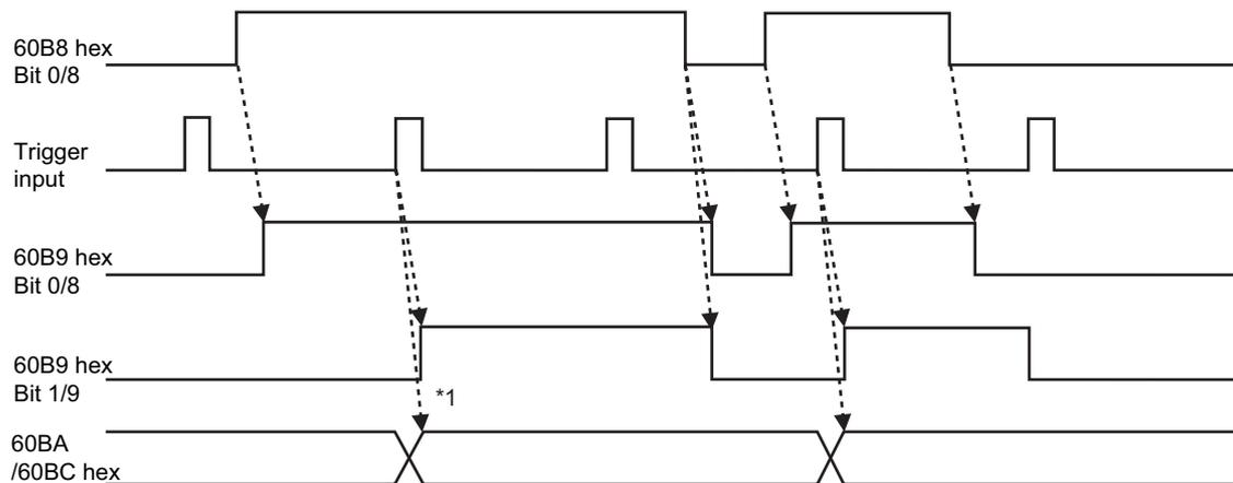
\*1 The delay time is several tens of microseconds between the trigger input and position latch. This value is a reference value. Design the operation with a margin.
