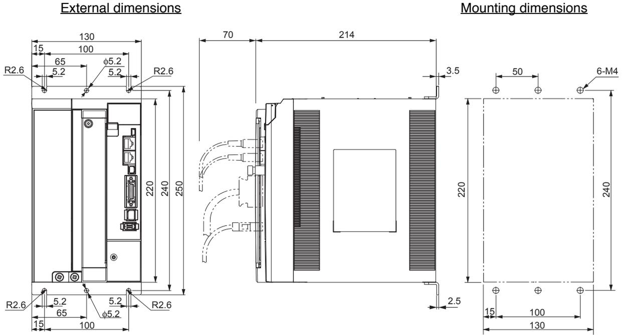
● **Front Mounting (Using Front Mounting Brackets)**
