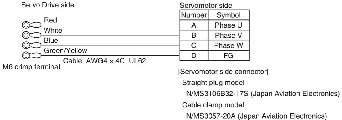
**Note 1** The cable length between the Servomotor and Servo Drive must be 50 m or less.
