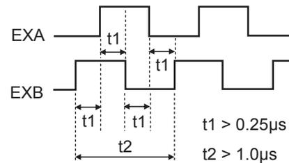
\*1 Connect external encoder signals to the serial interface (+EXS/-EXS) or 90° phase difference inputs according to the encoder type.
