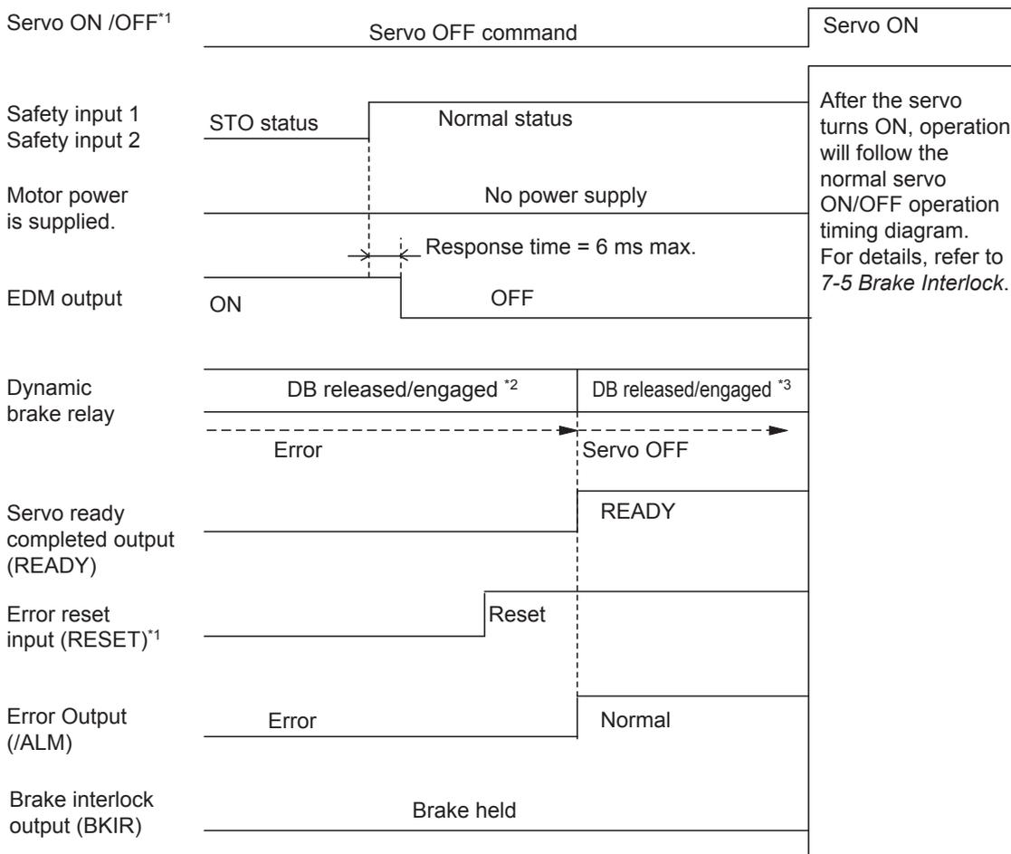
\*1 Make sure that servo ON input is turned OFF when you return the input signals of safety inputs 1 and 2 to ON. If an error exists in this state, be sure to clear the error when both safety inputs 1 and 2 have returned to ON state. Also, depending on the execution timing, an Other Error (Error No. 99.9) may occur. If this error (Error No. 99.9) occurs, turn OFF and then ON the power again.
