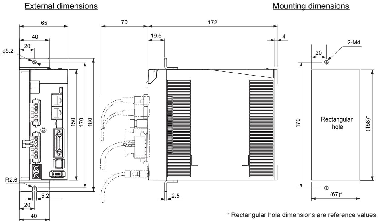
**Single-phase/3-phase 200 VAC: R88D-KN10H-ECT/-KN15H-ECT
