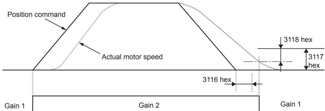
**Note** Whether there is a position command is determined by changes in the Target position (607A hex).
