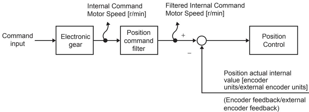
\*2 The position error is calculated for the command input after processing for the position command filter. The pulse position error or fully-closed position error is reversely converted to command input for application. The pulse position error or fully-closed error is the error for the position control input.
