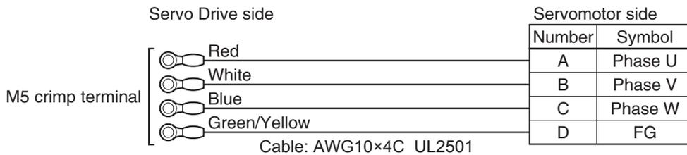
[Servomotor side connector]
