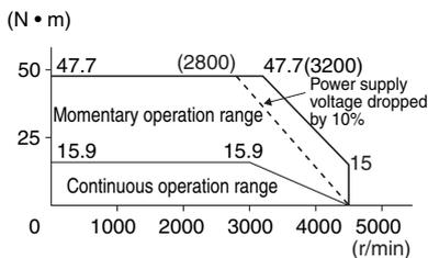
**Note 1** The continuous operation range is the range in which continuous operation is possible. Continuous operation at the maximum speed is also possible. However, doing so will reduce the output torque.
