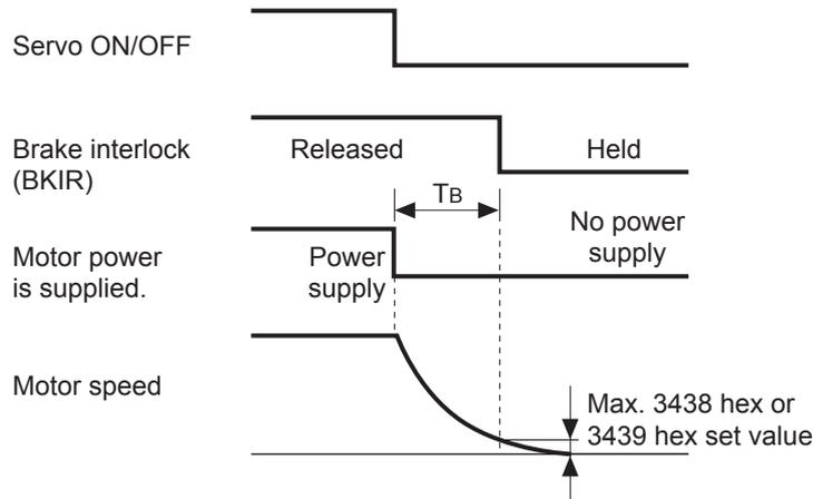
The time  $T_b$  in above drawing is either the brake timing during operation (i.e., the set value × 1 ms) or the time taken until it goes below the value set in the Brake Threshold Speed During Operation (3439 hex), whichever is shorter.
