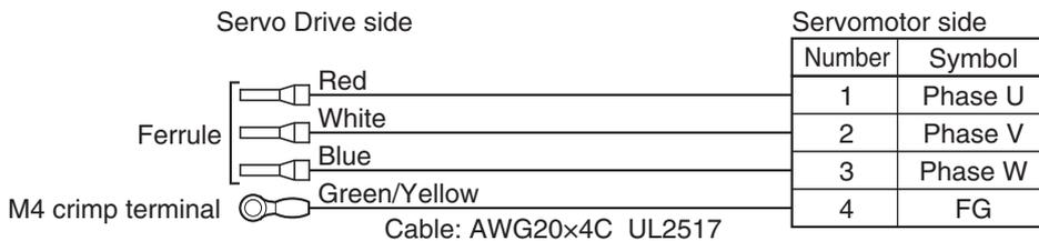
[Servomotor side connector]
