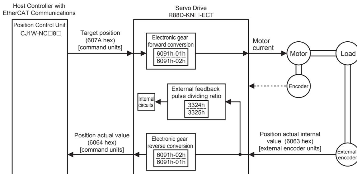
**Note** The electronic gear function is not supported for unit version 2.0. For the Servo Drives with unit version 2.0, set the electronic gear ratio to 1.1.
