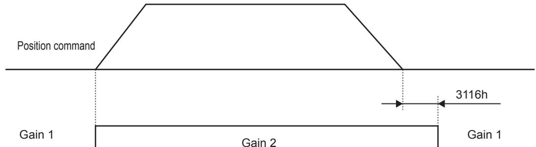
**Note** Whether there is a position command is determined by changes in the Target position (607A hex).
