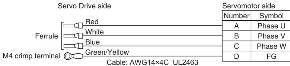
[Servomotor side connector]
