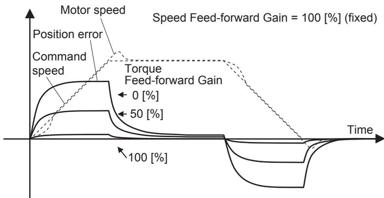
Torque feed-forward can reduce the position error in a range of constant acceleration/ deceleration.
