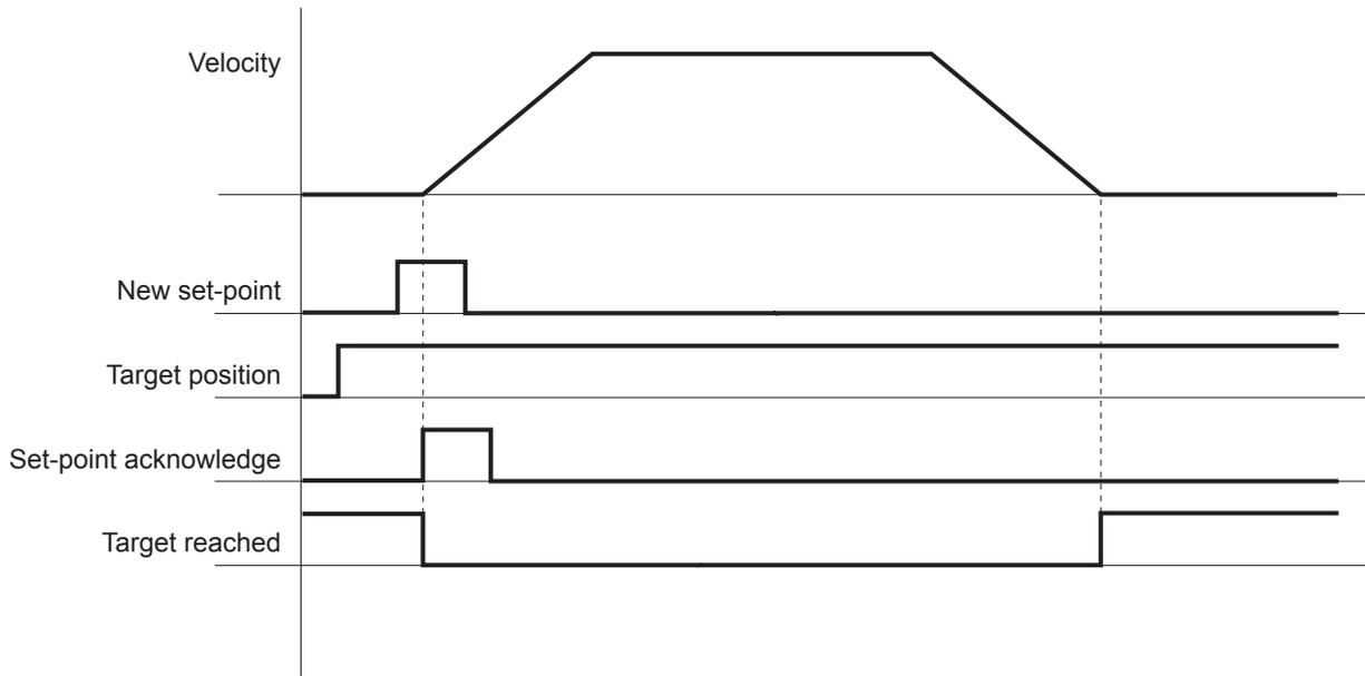
The Target value can be changed while PTP positioning is in progress.
