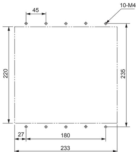
● Front Mounting (Using Front Mounting Brackets)
