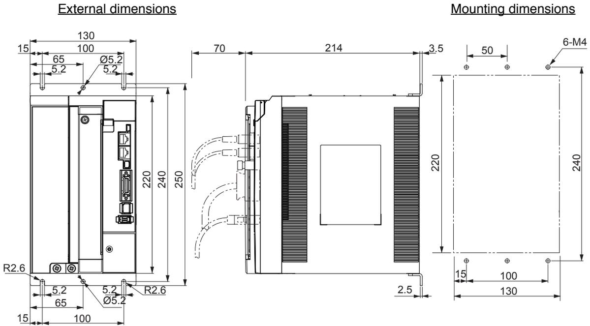
● **Front Mounting (Using Front Mounting Brackets)**
