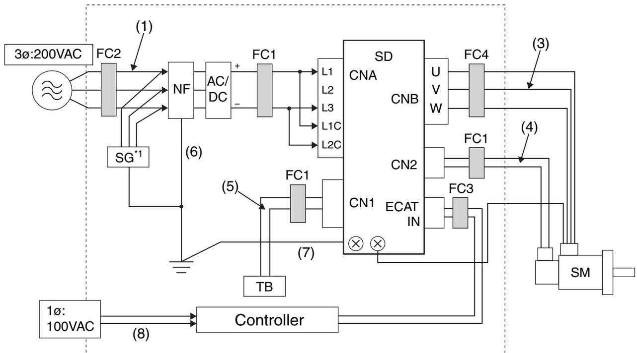
**Note** L1 and L3 are the main circuit power supply input terminals. Connect the positive wire to L1 and the negative wire to L3.
