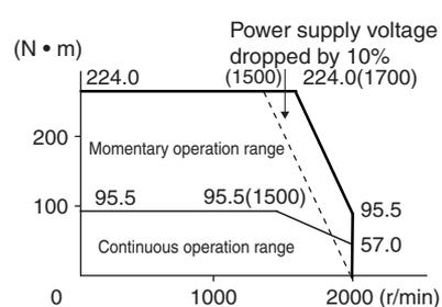
**Note 1** The continuous operation range is the range in which continuous operation is possible. Continuous operation at the maximum speed is also possible. However, doing so will reduce the output torque.
