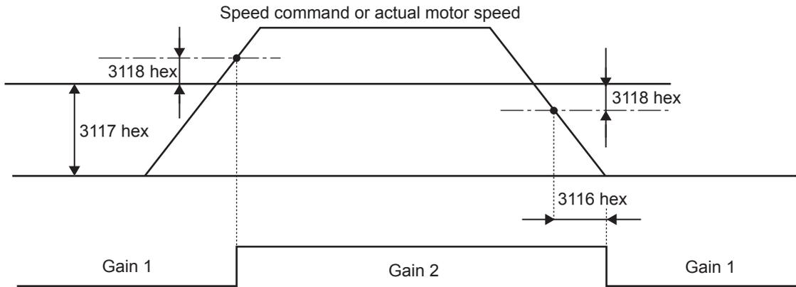
**Note** The “speed command” is the Motor Control Effort (401A hex) [r/min].
