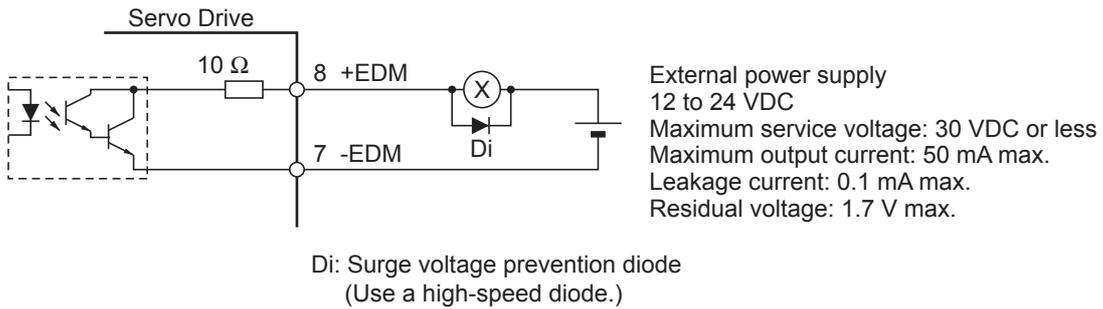
**Note** When driving a relay directly with an output signal, always insert a diode as shown in the above figure.
