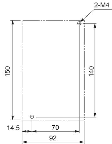
● **Front Mounting (Using Front Mounting Brackets)**
