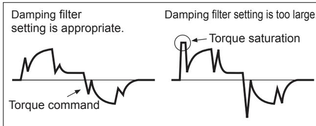
When setting the damping frequencies, reduce the setting if the torque become saturated and increase the setting to make operation faster. Normally 0 is set.
