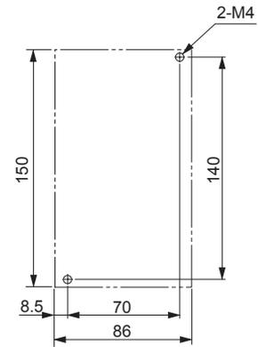
● **Front Mounting (Using Front Mounting Brackets)**
