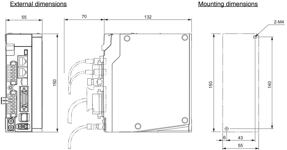
● **Front Mounting (Using Front Mounting Brackets)**
