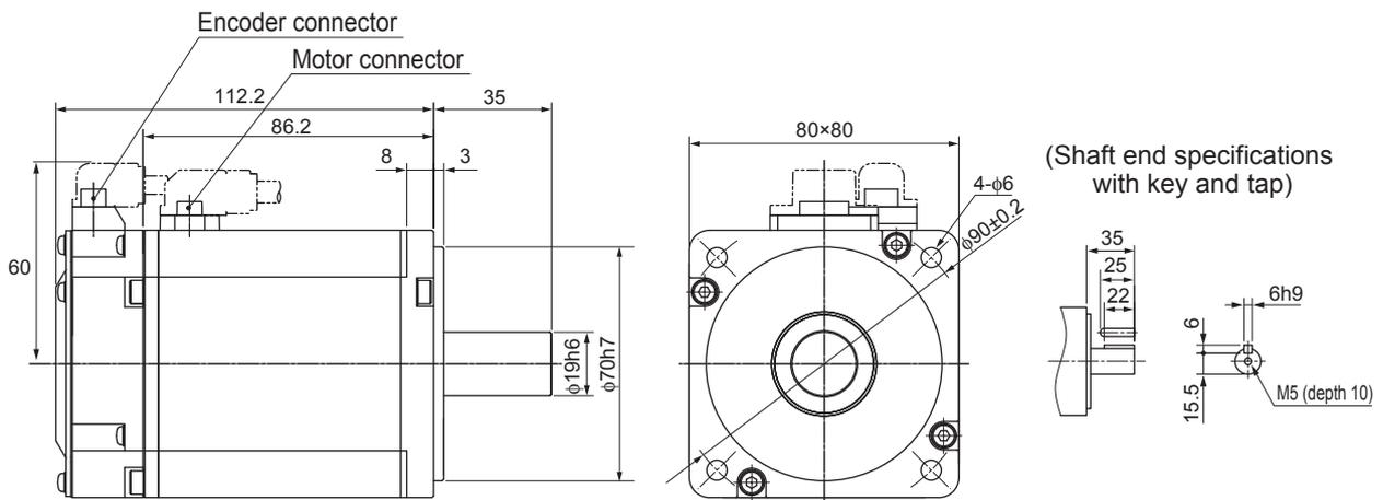
**Note** The standard models have a straight shaft. Models with a key and tap are indicated with S2 at the end of the model number.
