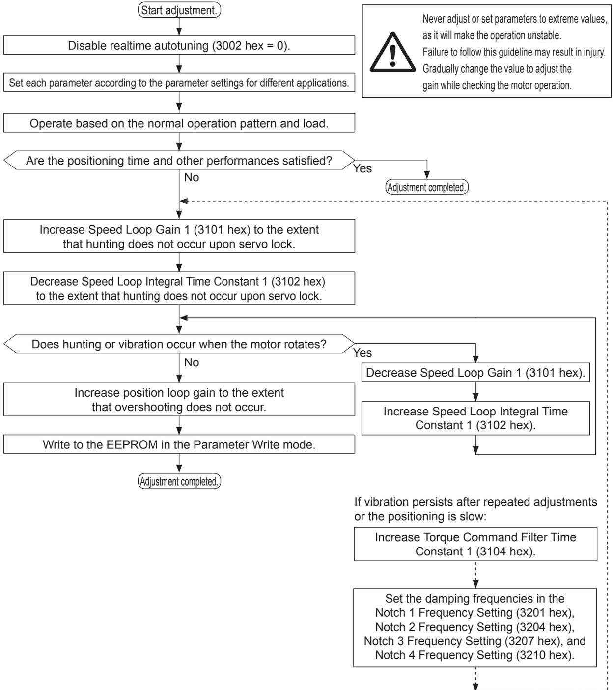
Never adjust or set parameters to extreme values, as it will make the operation unstable. Failure to follow this guideline may result in injury. Gradually change the value to adjust the gain while checking the motor operation.
