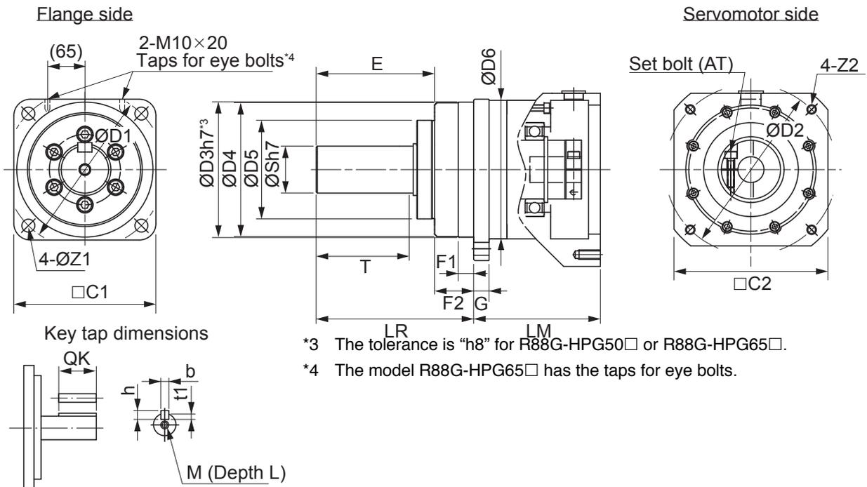
\*3 The tolerance is "h8" for R88G-HPG50□ or R88G-HPG65□.
