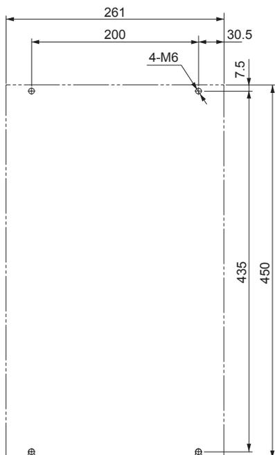
**3-phase 400 VAC: R88D-KN06F-ECT/-KN10F-ECT (600 W to 1.0 kW)**
