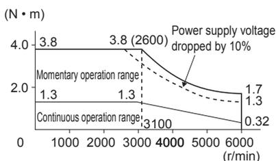
**Note 1** The continuous operation range is the range in which continuous operation is possible. Continuous operation at the maximum speed is also possible. However, doing so will reduce the output torque.
