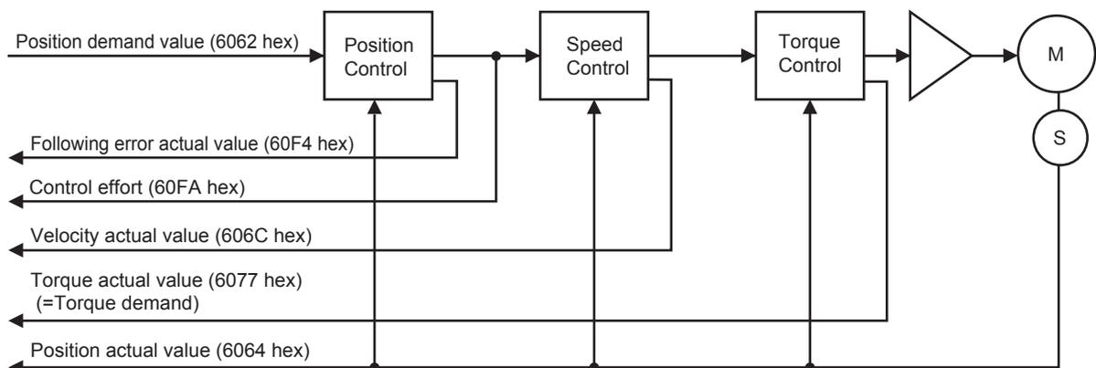
The following diagram shows the control function configuration of Profile position mode.
