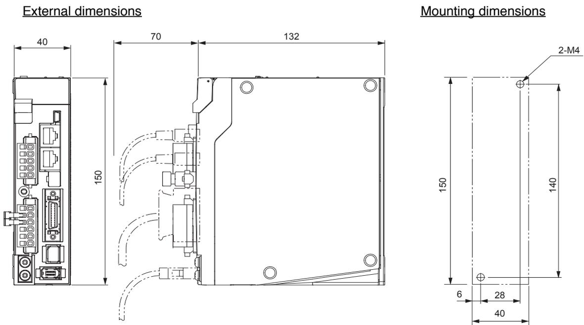
● Front Mounting (Using Front Mounting Brackets)
