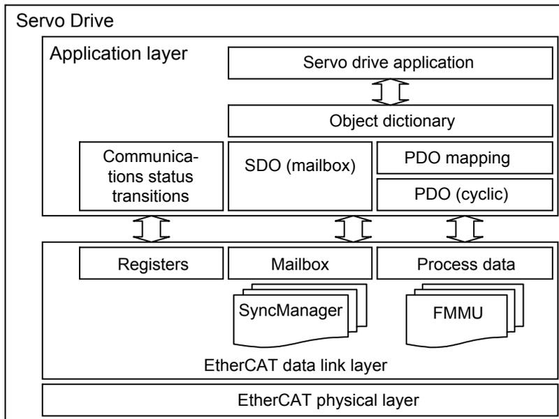
Normally, multiple protocols can be transmitted using EtherCAT. The IEC 61800-7 (CiA 402) drive profile is used for G5-series Servo Drives with Built-in EtherCAT Communications.
