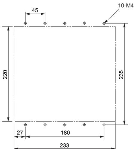
● **Front Mounting (Using Front Mounting Brackets)**
