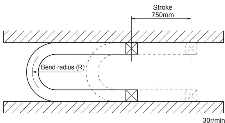
**Note** The following shows the stroke in some parts of the model.
