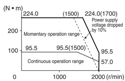
**Note 1** The continuous operation range is the range in which continuous operation is possible. Continuous operation at the maximum speed is also possible. However, doing so will reduce the output torque.
