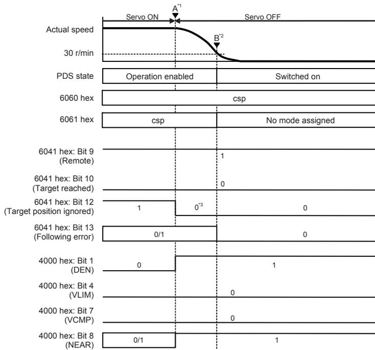
\*1 When the servo is turned OFF, a deceleration stop starts and 6061 hex continues to show the same mode as the mode of operation (csp) specified in 6060 hex.
