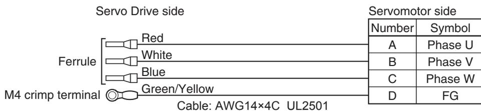
[Servomotor side connector]
