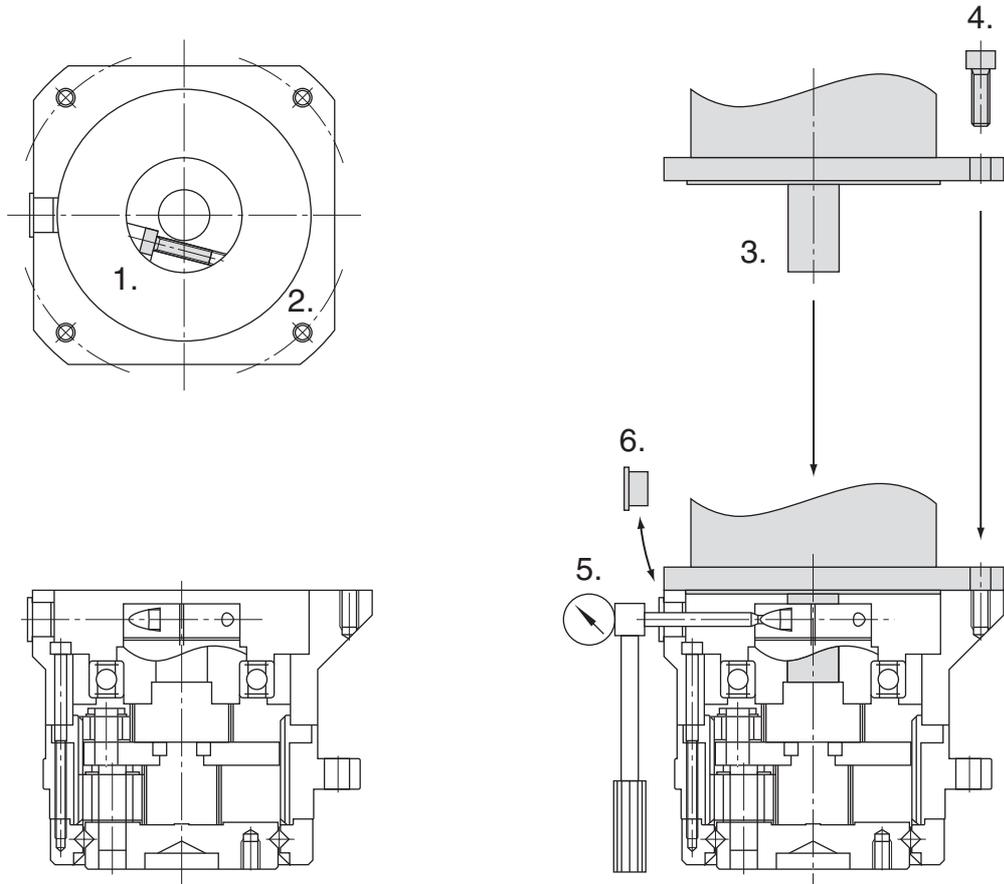
● **Installing the Reduction Gear into the machine.**
