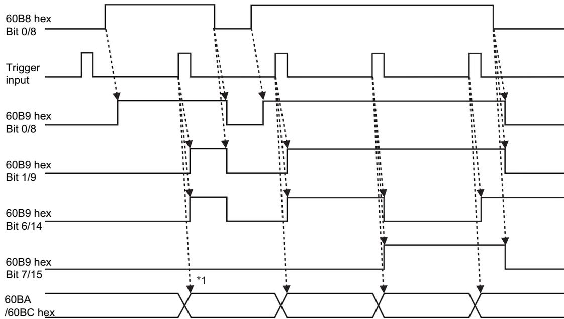
\*1 The delay time is several tens of microseconds between the trigger input and position latch. This value is a reference value. Design the operation with a margin.
