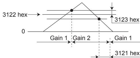
\*3 When the Gain switching command of EtherCAT communications (G-SEL) is 0, the gain switches to Gain 1. When the command is 1, the gain switches to Gain 2.
