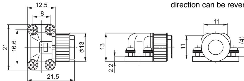
For the angle plug, cable pulling out direction can be reversed.
