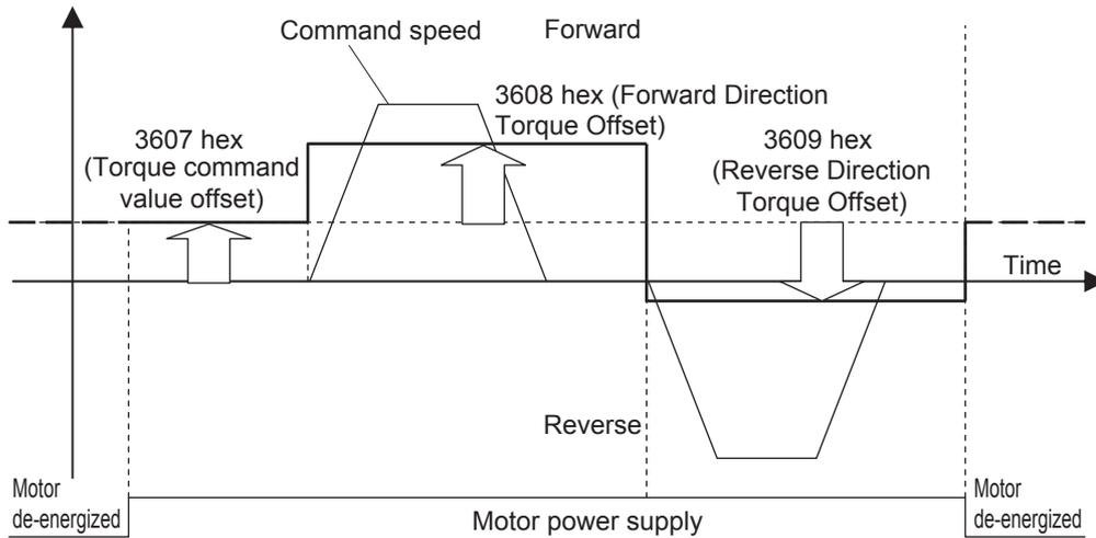
The Torque Command Value Offset (3607 hex) reduces the variations of positioning operations due to the movement directions when a certain amount of unbalanced load torque is always applied to the motor at the vertical axis by setting the torque command.
