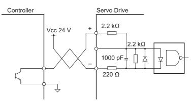
When an external power supply is used (at 200 kpps or lower) (+CW: 3, -CW: 4, +CCW: 5, -CCW: 6)
