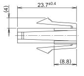
Connector housing model 172157-1 (Tyco Electronics AMP KK) Contact socket model 170366-1 (Tyco Electronics AMP KK) Panel mounting hole
