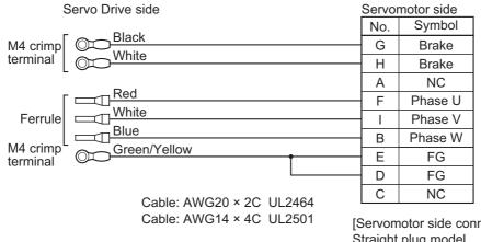
[Servomotor side connector] Straight plug model N/MS3106B20-18S (Japan Aviation Electronics) Cable clamp model N/MS3057-12A (Japan Aviation Electronics)
