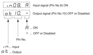
This indicates the status of the control input and output signals connected to CN1 pin.
