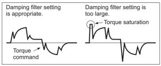
When Damping Frequency 1 (Pn214) is set, reduce this setting if torque saturation occurs or increase this setting to improve the operation speed. Normally 0 is set.
