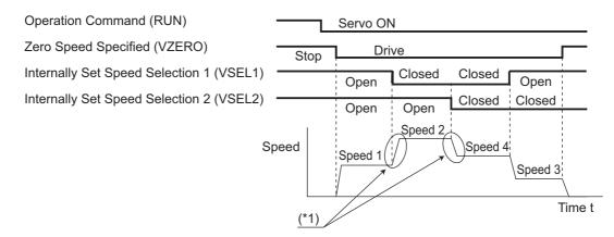
\*1 The acceleration time, deceleration time, and S-curve acceleration/deceleration time can be set in parameters Pn312, Pn313, and Pn314, respectively.
