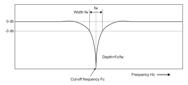
If mechanical resonance occurs, use this notch filter to eliminate resonance.
