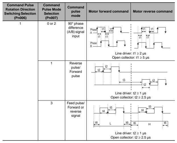
• Set the input pattern of the command pulses from the position controller to the Servo Drive.
