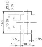
The applicable panel thickness is 0.8 to 2.0 mm.
