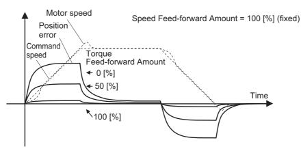
Torque feed-forward can reduce the position error in the range of constant acceleration/ deceleration.
