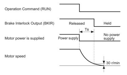
"TB" in the above figure is the setting time in Brake Timing During Operation or the time until the motor rotation speed falls to 30 r/min or lower, whichever is shorter.
