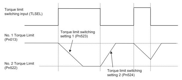
If the No. 1 Torque Limit (Pn013) or No. 2 Torque Limit (Pn522) value is changed from the front panel or CX-Drive, the rate of change setting is ignored and the new torque limit value is applied immediately.
