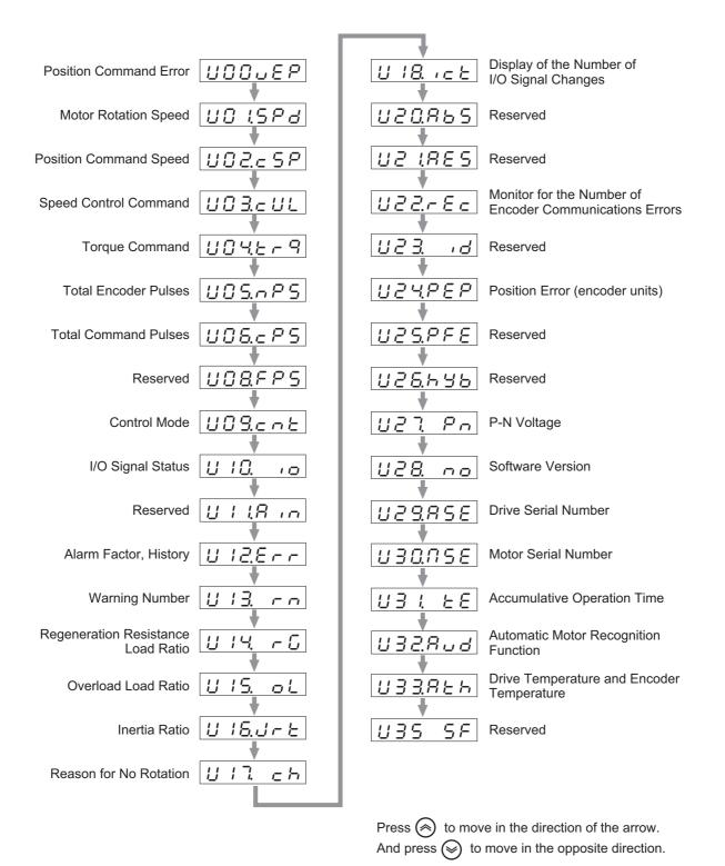
• The display shows the motor rotation speed when the power supply is turned ON for the first time after purchase. To change the display that appears when the power supply is turned ON, change the value set in Default Display (Pn528). For details, refer to Pn528 *Default Display* on page 7-53.
