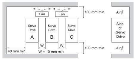
• If the mounting surface of the Servo Drive is coated, remove the coating to allow electrical conduction. If you make your own mounting bracket, we recommend that you apply electrically conductive plating.
