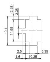
\*1 The applicable panel thickness is 0.8 to 2.0 mm.
