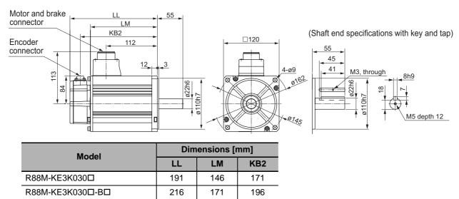
**Note** The standard models have a straight shaft. Models with a key and tap are indicated with S2 at the end of the model number.
