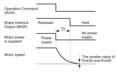
"TB" in the above figure is the setting time in Brake Timing During Operation (Pn438) (set value  $\times$  1 ms) or the time until the motor rotation speed falls to the setting speed or lower in Brake Release Speed Setting (Pn439), whichever is shorter.
