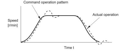
• If the position loop gain is low, positioning completion speed becomes slow.
