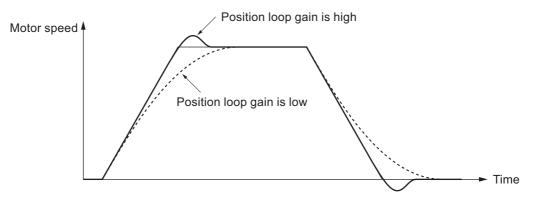
• If the speed loop gain and position loop gain are optimally set, the motor operation delays 2/Kp for acceleration and 3/Kp for deceleration in response to command input.
