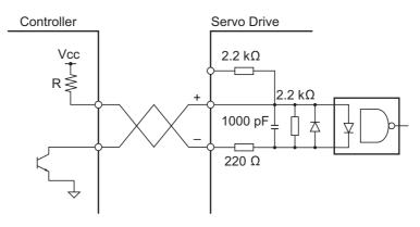
Select an appropriate Current Limit Resistor (R) for Vcc.
