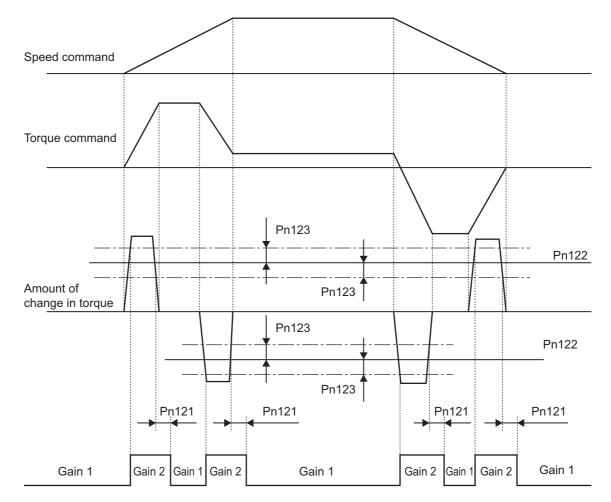
Gain Switching Mode = 5 or 9: Switching by Speed Command or Actual Motor Speed
