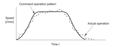
• If the speed loop integral time constant is high, the response is delayed. The servo rigidity becomes weak.
