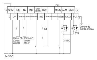
\*1 CW and CCW limit input signals can also be input to an input unit. For CJ2M, the CW and CCW limit input signals function with the following signals. CW: A540.08/CCW: A540.09 (Pulse output 0), CW: A541.08/CCW: A541.09 (Pulse output 1) Therefore, in ladder programming, use the actual input as CW and CCW limit input signals to output the following flag.
