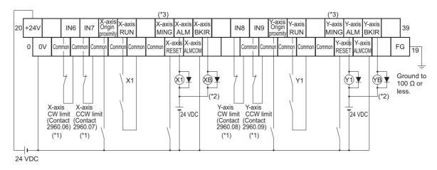
\*1 CW and CCW limit input signals can also be input to an input unit. For CJ2M, the CW and CCW limit input signals function with the following signals. CW: A540.08/CCW: A540.09 (Pulse output 0), CW: A541.08/ CCW: A541.09 (Pulse output 1) Therefore, in ladder programming, use the actual input as CW and CCW limit input signals to output the following flag.
