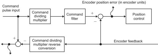
Position command error (in command units)/ Command feedback pulse error (in command units)
