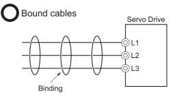
• Separate power supply lines and signal lines when wiring.
