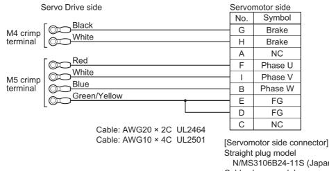
N/MS3106B24-11S (Japan Aviation Electronics) Cable clamp model N/MS3057-16A (Japan Aviation Electronics)
