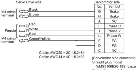
Straight plug model N/MS3106B20-18S (Japan Aviation Electronics) Cable clamp model N/MS3057-12A (Japan Aviation Electronics)
