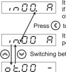
It is possible to change the signal number if the decimal point is located on the right of the signal number.
