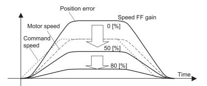
The position error in the constant speed range becomes smaller as the speed feed-forward gain increases.
