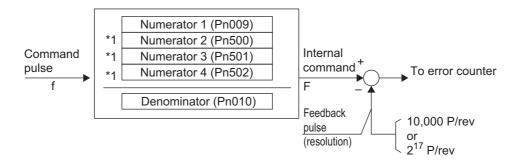
\*1 The selection of second to fourth numerators is made based on the Electronic Gear Switching 1 and 2 (GESEL1 and GESEL2) settings.
