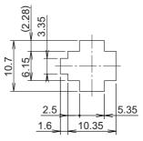
The applicable panel thickness is 0.8 to 2.0 mm.
