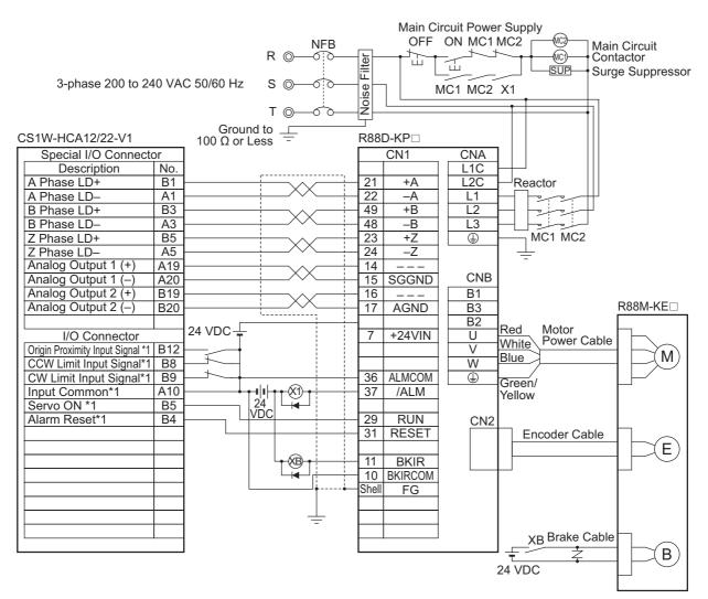
\*1 The I/O signals for the HCA12/22 vary depending on the allocations in the internal relay area. Change the wiring according to the allocations.
