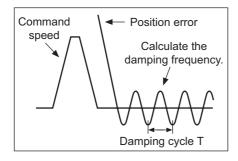
• The damping frequency in the figure is calculated with the following formula:
