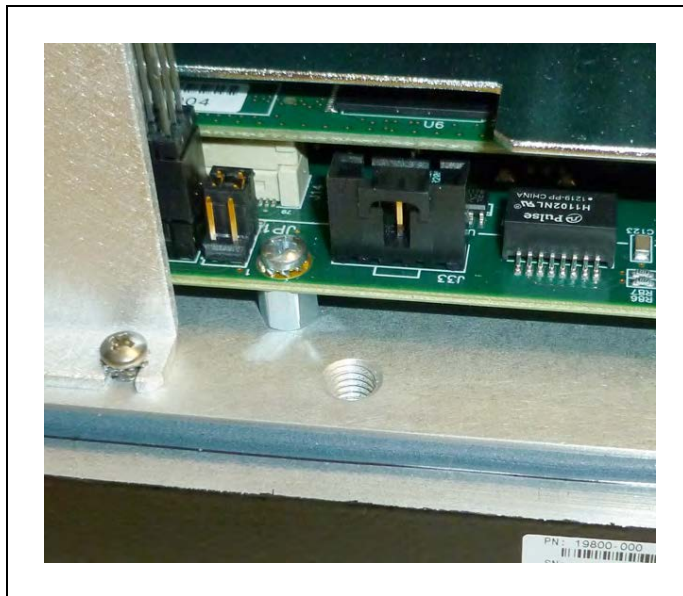
Figure 6-11. Ground Screw Hole on eAIB Chassis
