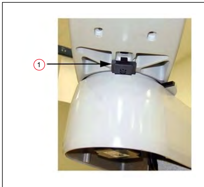
Figure 7-23. (1) Fixed Hardstop Block for Joint 2
