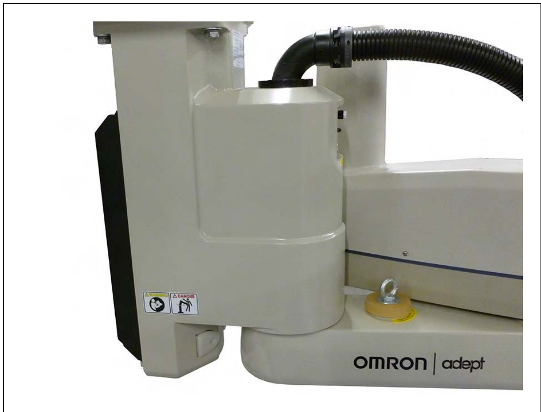
Figure 6-2. Location of Read Manual and Impact Warning Label (Inverted Model Shown).
