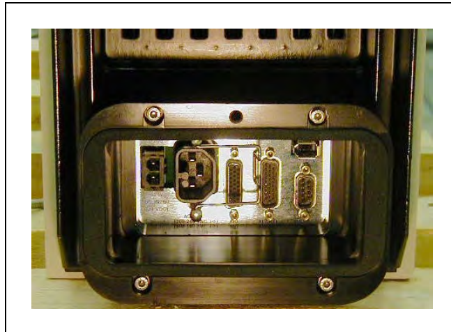
Figure 9-3. Cable Seal Housing Installed
