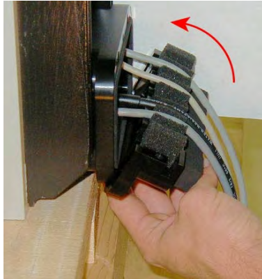
Figure 9-4. Installing Lower Flange
