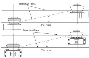
When installing the OS32Cs side by side, it is more effective to set their mounting heights differently. When adjusting the OS32C tilted, it may be more effective to adjust the OS32C downward depending on the condition of the outside light source (natural light or halogen light).
