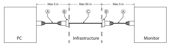
The following table lists the recommended cables and materials for the NY Monitor Link cable applications up to 100 m.
