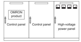
**Example of Poor Equipment Arrangement**
