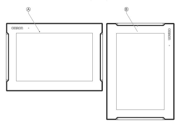
Do not install the Industrial Monitor in any of the following orientations.
