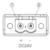
The pin layout represents the power connector on the Industrial Monitor.
