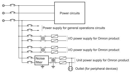
Power Supply System Diagram
