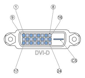
The pin layout represents the DVI connector on the Industrial Monitor. Pin numbers increase from left to right for every row.
