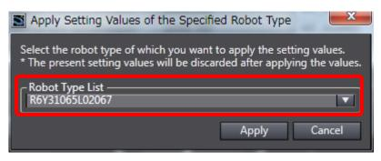
Click the **Apply** Button to apply the kinematics and workspace setting values of the selected robot type to the *Value* Column in the 3D Equipment Model Creation Wizard.
