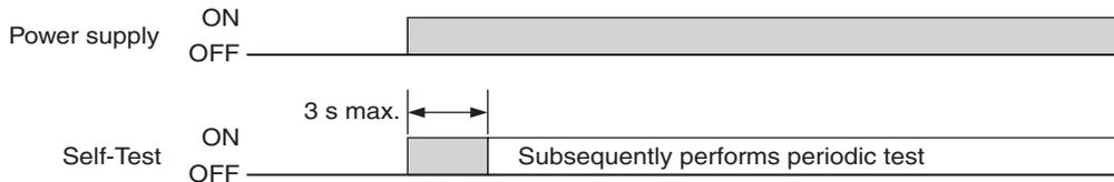
If an error is found in the Self-Test, the F3SG-SR/PG enters the LOCKOUT state, keeps the safety outputs in the OFF state, and indicates the error at the same time.
