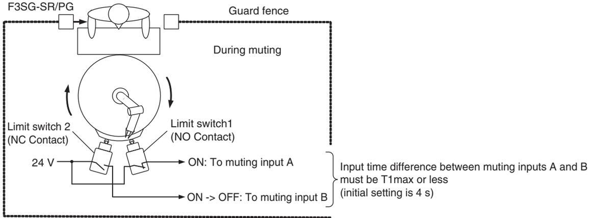
If the duration between when the muting input A is turned ON from the OFF state and when the muting input B is turned OFF from the ON state is within  $T1_{max}$  [ s ], the safety function of the F3SG-SR/PG is disabled.
