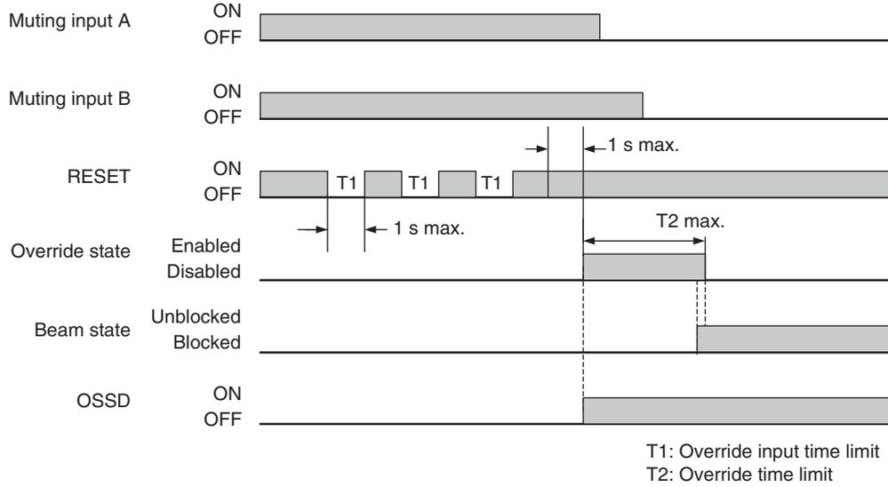
Note. In this timing chart, the OVERRIDE state ends when the F3SG-SR/PG receives light.
