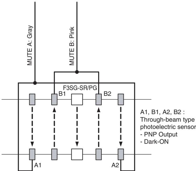
Using an NO contact type switch as a muting sensor (PNP)
