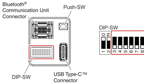
For details of the channels, refer to 3-5. *DIP Switch on Intelligent Tap.*
