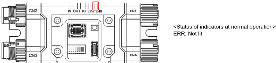
If the ERR indicator is ON, turn off power of the Intelligent Tap and F3SG-SR/PG, make sure that the wiring is proper, and go back to step 3 to perform the steps again.
