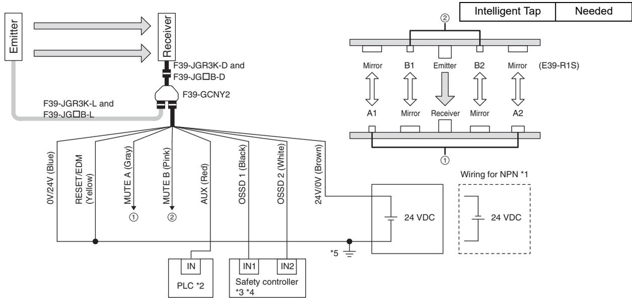
PLC: Programmable logic controller (Used for monitoring only. NOT related to safety system.)
