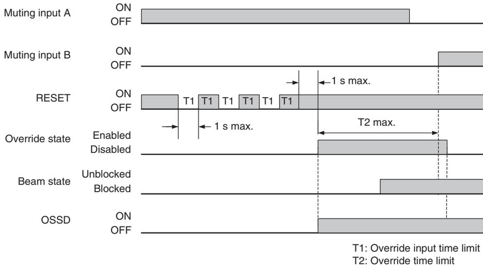
Note. In this timing chart, the OVERRIDE state ends when the muting input A is OFF and the muting input B is ON.
