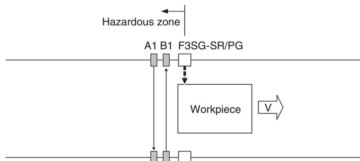
The workpiece has completely passed the muting sensor B1 and the sensor is turned OFF. The F3SG-SR/PG disables its safety function if it is within the exit-only muting delay time.
