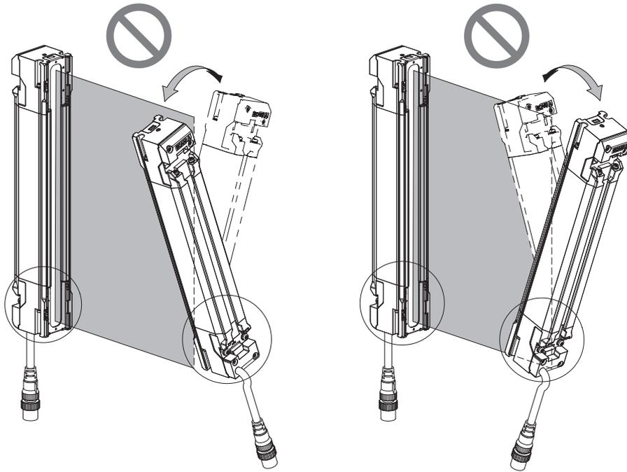
The detection surfaces of the emitter and receiver are not in parallel to each other.
