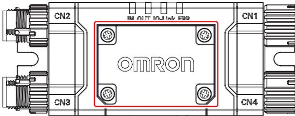
2. If a cable is not attached to CN3, use the torque wrench XY2F-0004 to attach the accessory waterproof cover (for plug). (Recommended tightening torque for waterproof cover (for plug): 0.39 to 0.49N•m)
