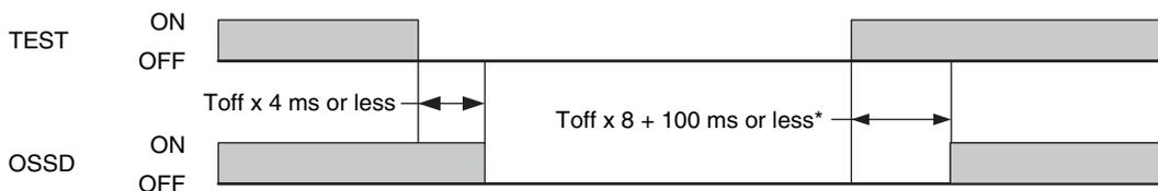
\* Toffx8 + 100 ms or less is the value when the Optical Synchronization is used. When the Wired Synchronization is used, the time is Toff × 8 ms or less.
