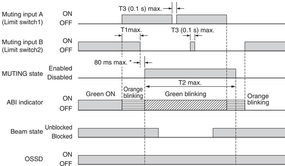
\* 102 ms max. when the Intelligent Tap is connected to the F3SG-SR.
