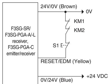
S1: Lockout or interlock reset switch
