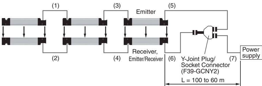
Maximum cable extension (Load condition: Safety outputs 1 and 2: 60 mA, Auxiliary output : 60 mA)
