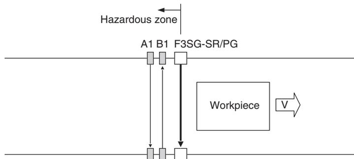
A workpiece has passed the F3SG-SR/PG's detection zone. When the muting end wait time: T4 (1 s: configurable) passes after the F3SG-SR/PG is unblocked, the MUTING state is released.
