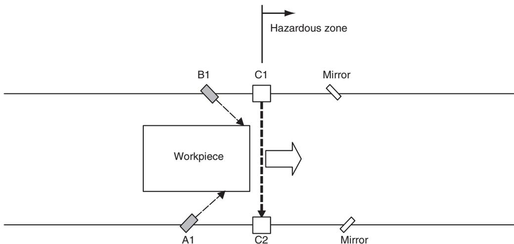
When the muting sensors A1 and B1 are turned ON in this order, the F3SG-SR enters the MUTING state. In this state, the safety function of F3SG-SR/PG C1 and C2 is disabled.
