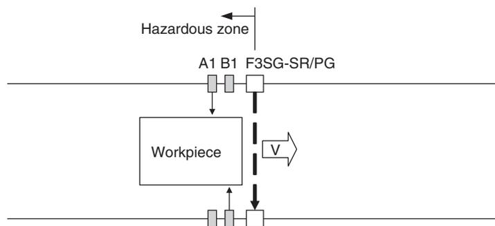
When the muting sensors A1 and B1 are turned ON in this order, and the MUTING state is enabled. In this state, the safety function of F3SG-SR/PG is disabled.
