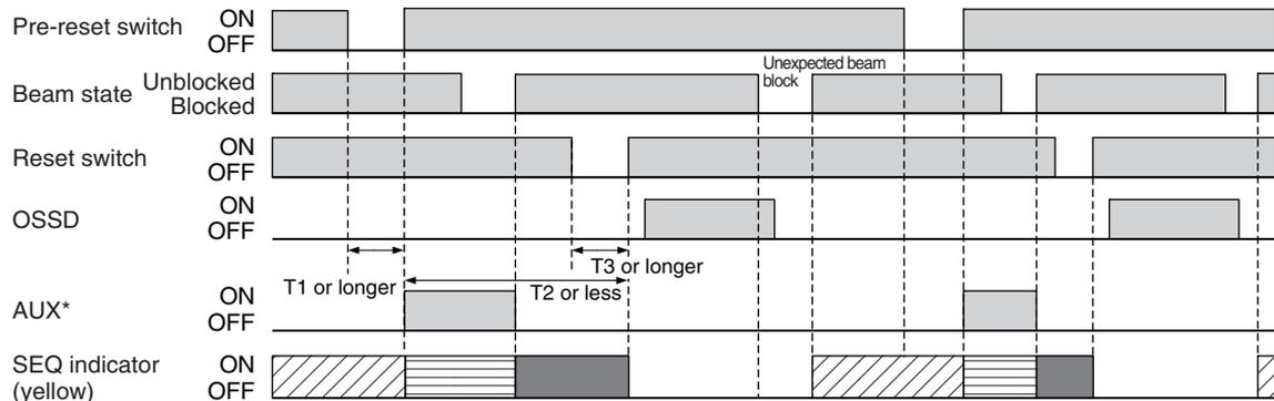
T1: Minimum pressing time of pre-reset switch. Configurable from 100 to 500 ms in 100-ms increments. T3 = T1
