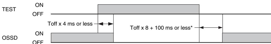
Emission stops when connected to 24 VDC:
