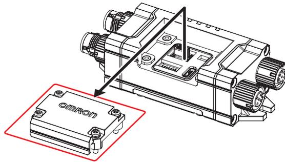
3. Set the DIP Switch position 1 ON and position 2 OFF.
