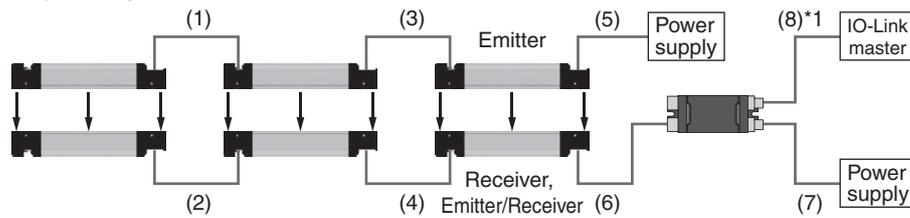
Maximum cable extension (Load condition: Safety outputs 1 and 2: 60 mA, Auxiliary output : 60 mA)
