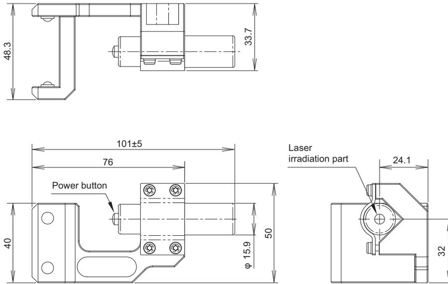
Material: Aluminum (Laser module case)
