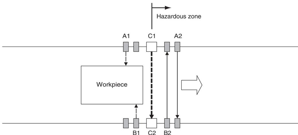
When the muting sensors A1 and B1 are turned ON in this order, MUTING starts. In this state, the safety function of F3SG-SR/PG C1 and C2 is disabled.
