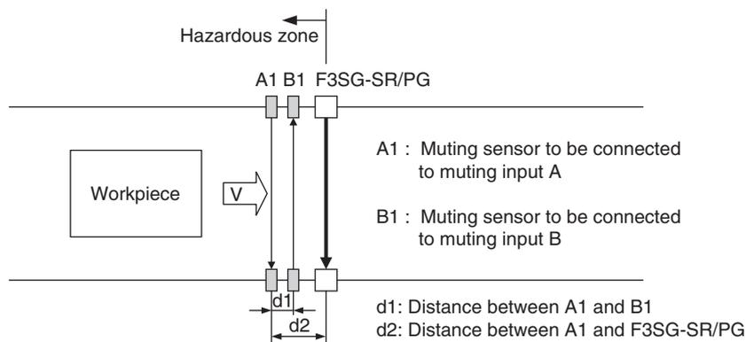
All muting sensors are turned OFF and the safety function of the F3SG-SR/PG is working.
