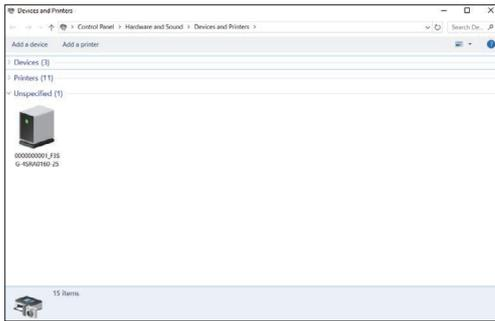
4. When selecting the [Hardware] tab, the screen below is displayed that indicates a COM port. In this example, the device “000000001\_F3SG-4SRA0160-25” is set to COM7.
