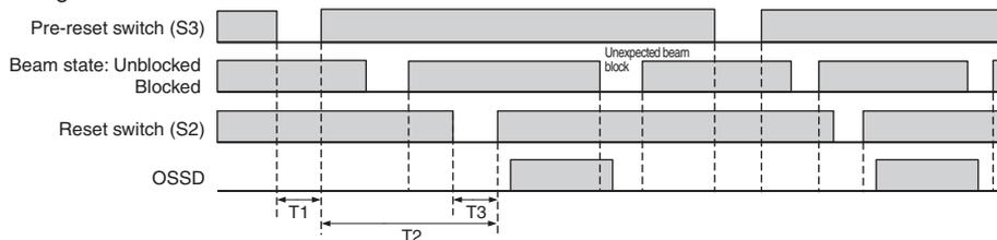
T1: Minimum pressing time of pre-reset switch. Configurable from 100 to 500 ms in 100-ms increments.
