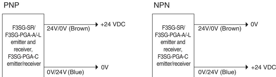
The F3SG-SR is set to PNP when the 24V/0V line (brown) is connected to +24 VDC and the 0V/24V line (blue) to 0 V.
