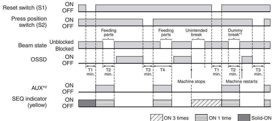
T1: Minimum pressing time of reset switch, configurable by 100 ms in a range of 100-500 ms
