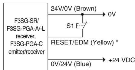
S1: Lockout or interlock reset switch
