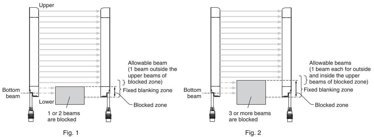
When beams including the top beam are blocked:
