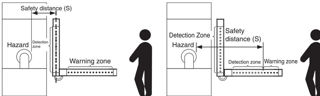
Refer to 5-1-2. *Safety Distance* for more information on safety distance calculations for orthogonal and parallel approaches.
