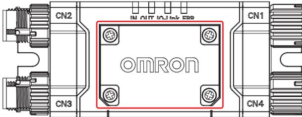
2. If a cable is not attached to CN3, use the torque wrench XY2F-0004 to attach the accessory waterproof cover (for plug).
