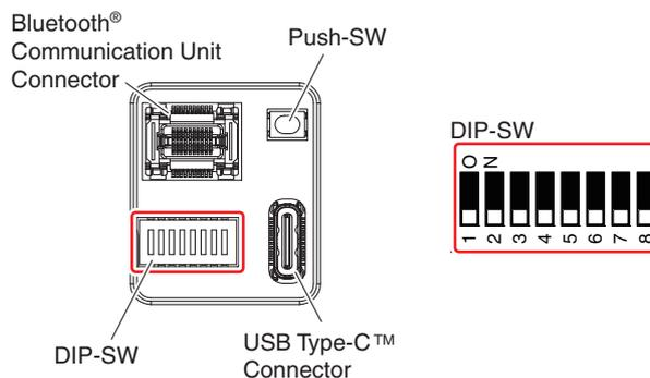
4. If the intelligent tap is not connected yet, connect it to F3SG-SR/PG. Refer to the chart in 3-10-1. *Setting F3SG-SR/PG with DIP Switch, ■Step 5.* to make sure that the system has the configuration with intelligent tap.
