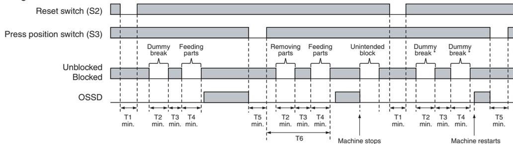
T1: Minimum pressing time of reset switch. Configurable from 100 to 500 ms in 100-ms increments by SD Manager 3.
