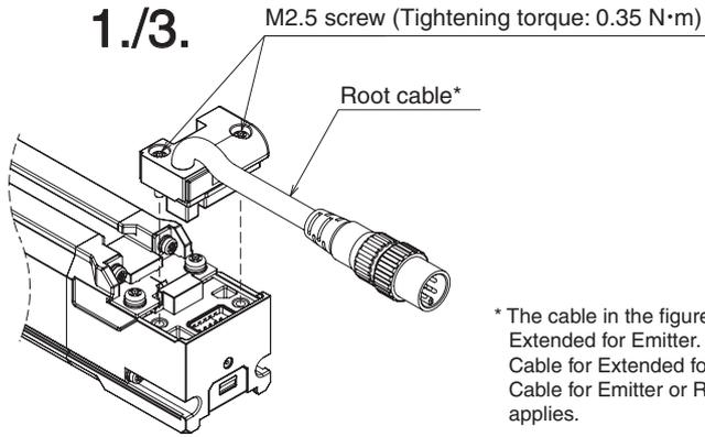
\* The cable in the figure is a Root-Plug Cable for Extended for Emitter. For connecting a Root-Plug Cable for Extended for Receiver and Root-Straight Cable for Emitter or Receiver, the same method applies.
