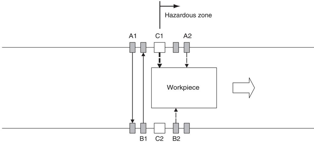
The muting sensors A1 and B1 are turned OFF but A2 and B2 are ON, so the MUTING state is still maintained. The OSSD 1 and 2 are turned ON.
