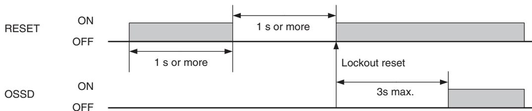
The table below shows the relation between the ON/OFF states and external lines.
