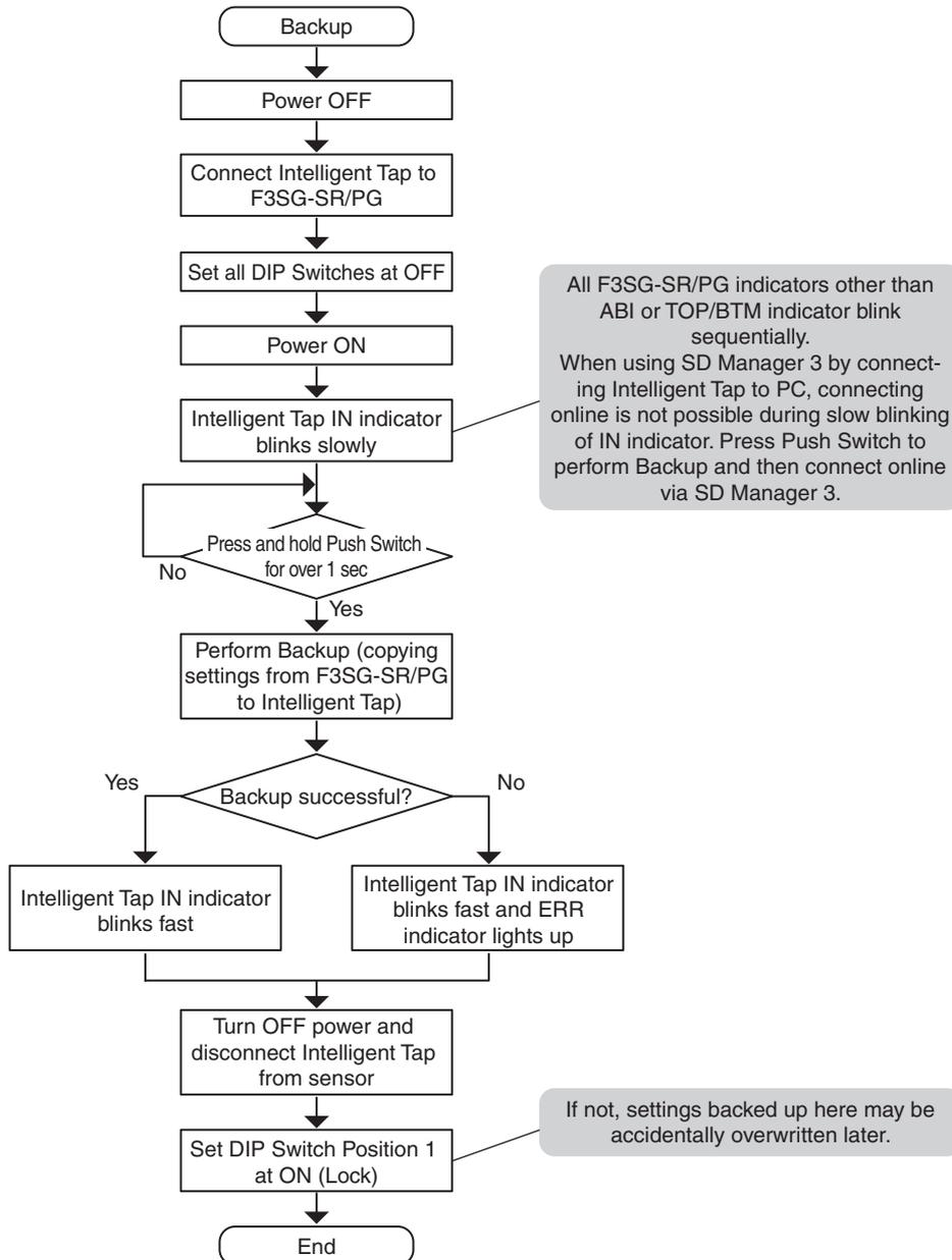
To run the Intelligent Tap while being connected to the F3SG-SR/PG, you must save the F3SG-SR/PG's settings in the Intelligent Tap by the backup operation. After performing the Backup, set the DIP Switch Position 1 at ON (Lock) and connect the Intelligent Tap to the F3SG-SR/PG.
