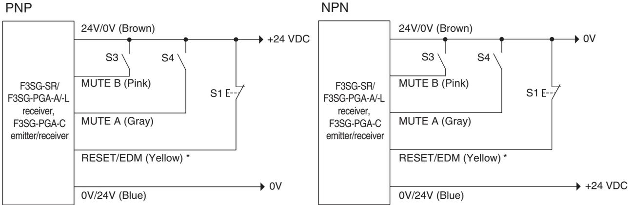
S1: Lockout/interlock reset switch or override switch or override cancel switch
