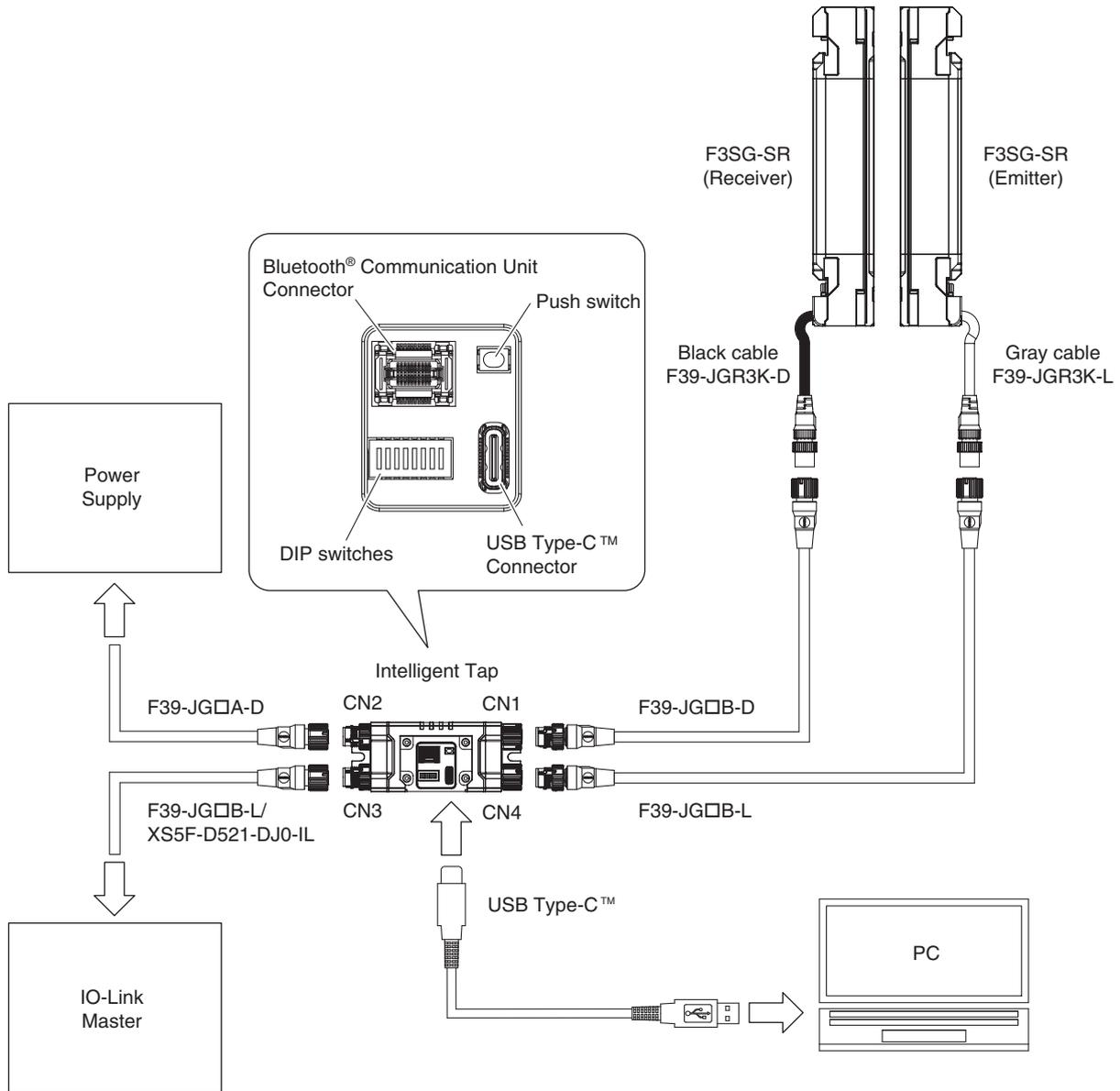
If you do not want to permanently install an Intelligent Tap and use an Intelligent Tap as needed, please temporarily change the wiring as shown below.
