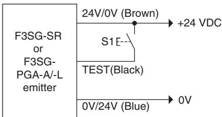
S1: Test switch (Connect the line to 0 V if this switch is not required.)
