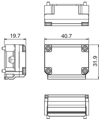
Material: PBT resin (Body parts)
