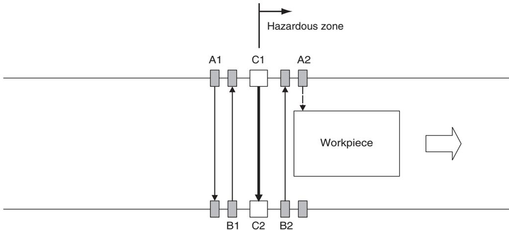
The muting sensor B2 is turned OFF, the Muting state is released, and the safety function of the F3SG-SR/PG C1 and C2 is enabled.
