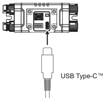
7. Connect the USB cable to the PC and run SD Manager 3.
