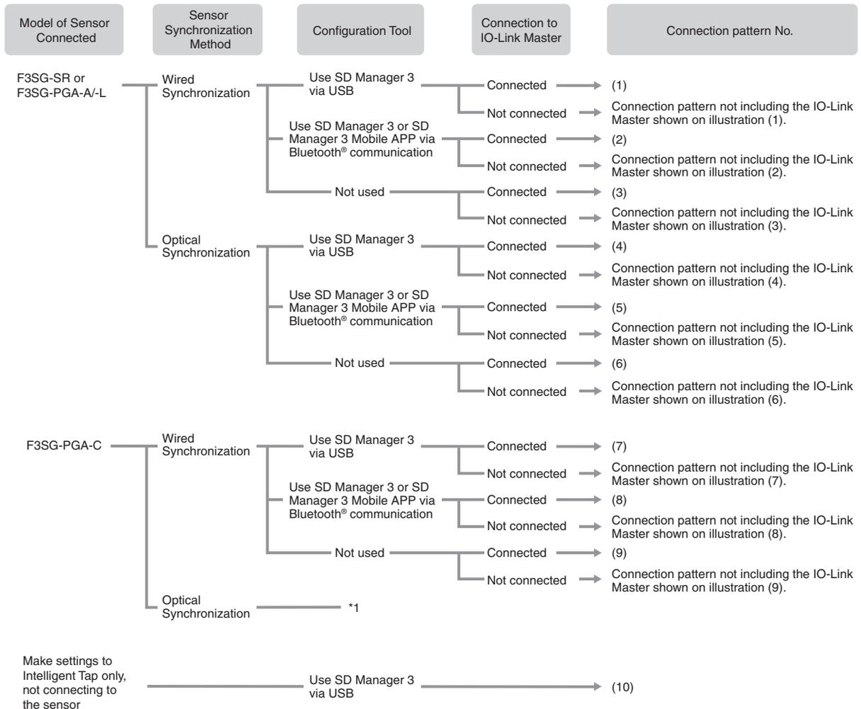
\*1 By connecting the emitter/receiver of F3SG-PGA-C with the Intelligent Tap, the product operates in the Wiring Synchronization. To connect a F3SG-PGA-C product operating in the Optical Synchronization with SD Manager 3, connect the Intelligent Tap temporarily, and remove it after settings are made. For further information on the operation in the Wiring Synchronization and Optical Synchronization of F3SG-PGA-C, refer to 2-3. *Mutual Interference Prevention*.
