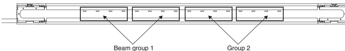
For example on the figure above, if even one of the beams in beam group 1 is blocked, the ABI indicators of that group are illuminated in red. When all the beams in that group are unblocked, the ABI indicators are turned OFF.
