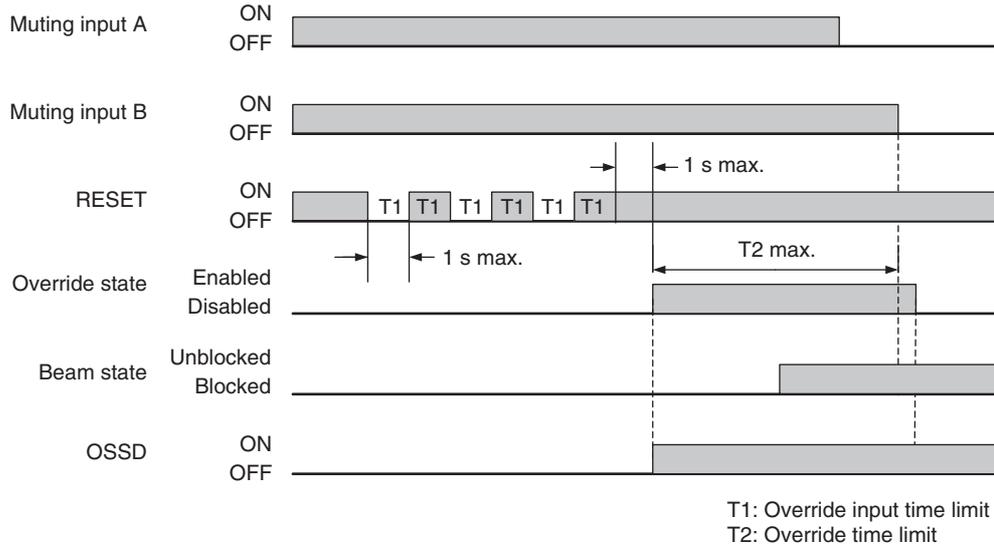
Note. In this timing chart, all muting sensors switched to OFF ends the OVERRIDE state.
