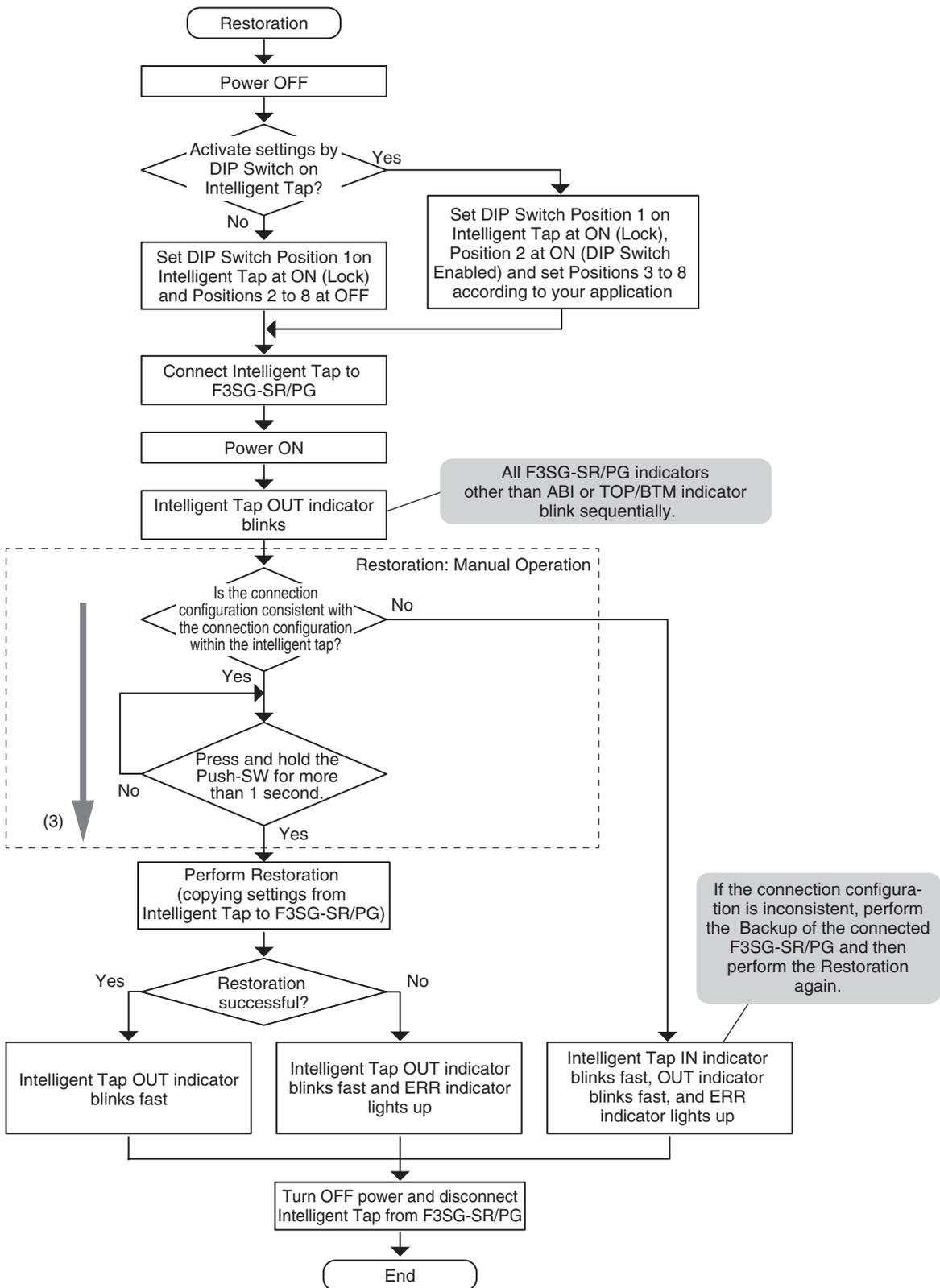
If the sensor configuration (model and cascading) in the Intelligent Tap corresponds with that of the actual one, the Restoration is automatically performed.(1)
