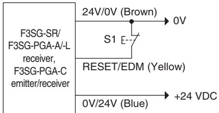
S1: Lockout or interlock reset switch
