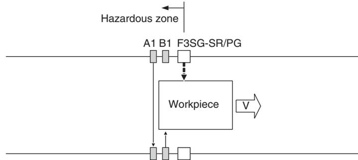
The workpiece has completely passed the muting sensor A1 and the sensor is now in the OFF state. In the Standard Muting mode, the Muting state is released here. In the Exit-Only Muting mode, the F3SG-SR/PG's safety function is disabled for the exit-only muting delay time: T5.
