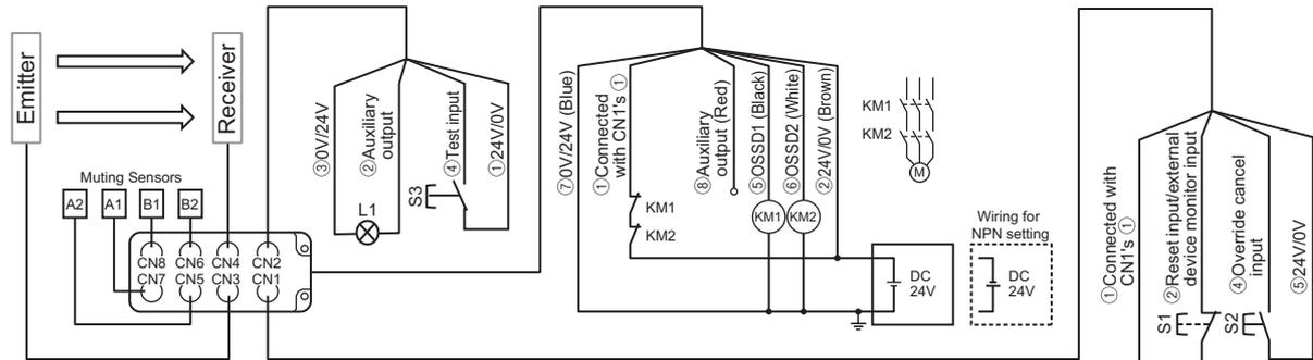
S1: Lock out/interlock reset/override switch
