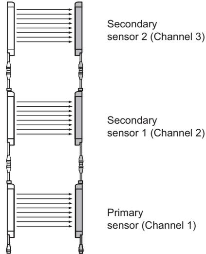
Properly connect an emitter to another emitter, and a receiver to another receiver, as shown below.
